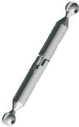
Figure 21. Model of adaptronic strut by CAD data
