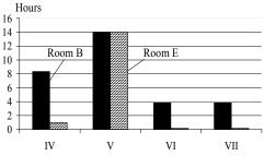
Figure 6: Frequencies of different sensations in room B (east) and E (west) during summer 2003 (May 1<sup>st</sup> to September 30<sup>th</sup>) with only considering the hours when the temperature limit was exceeded during the attendance time: (IV) windows opened manually; (V) shading system opened; (VI) shading system closed at least 70% and window opened.
