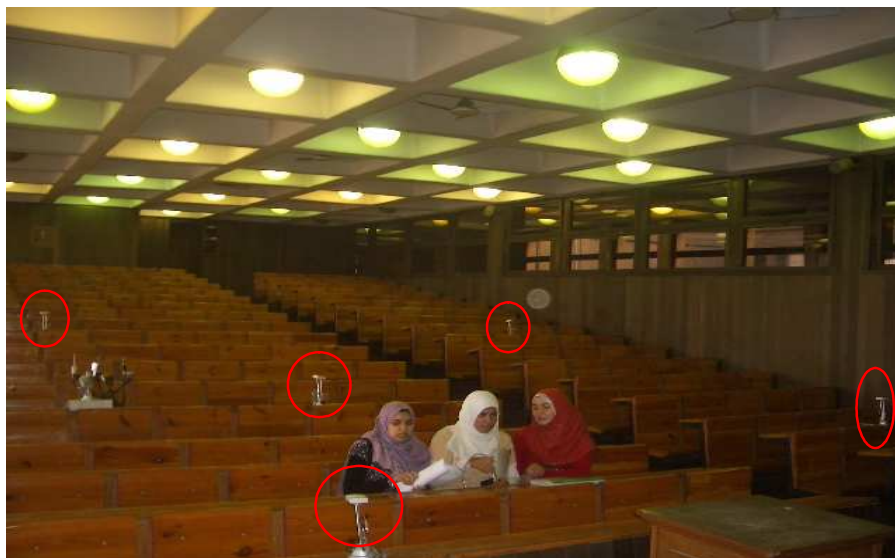
Figure (5): The data Loggers distributed over the whole space and their heights adjusted to the level of the students' heads.
