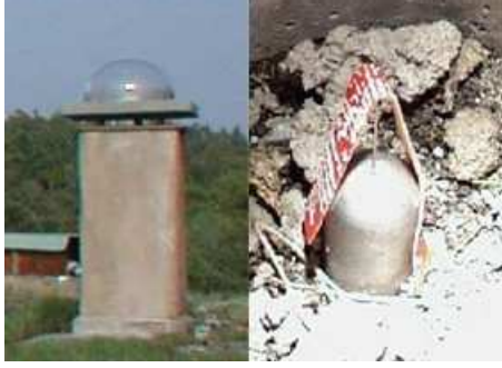
Figure 1. IGS-reference point (right) in the IGS-monument (left).
