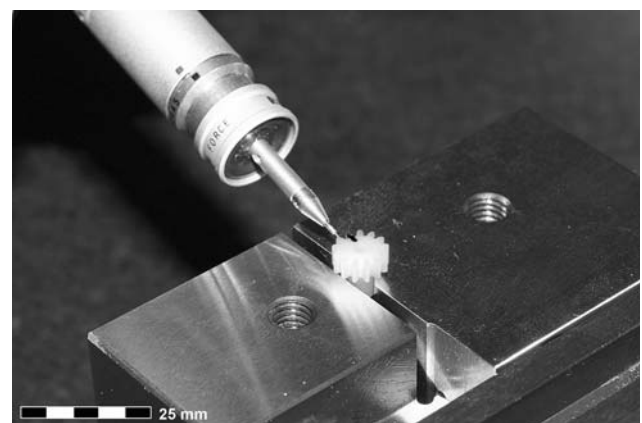
Fig. 3 Gearwheel measuring via tactile coordinate measuring machine
