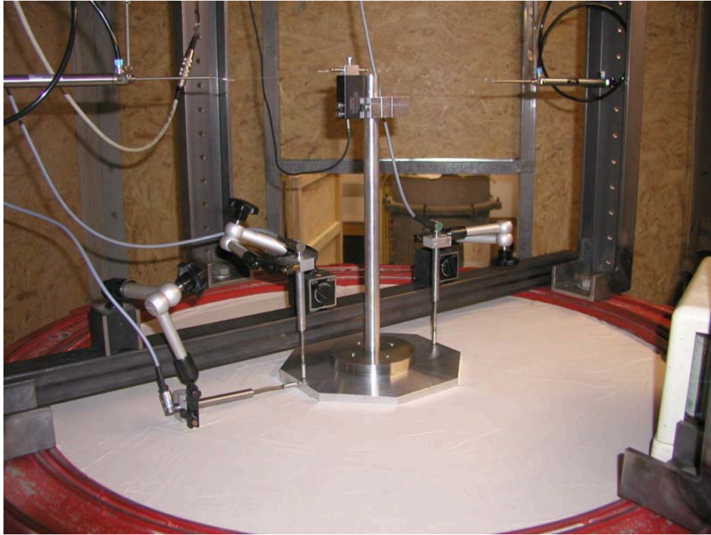
(a) View on model foundation and instrumentation
