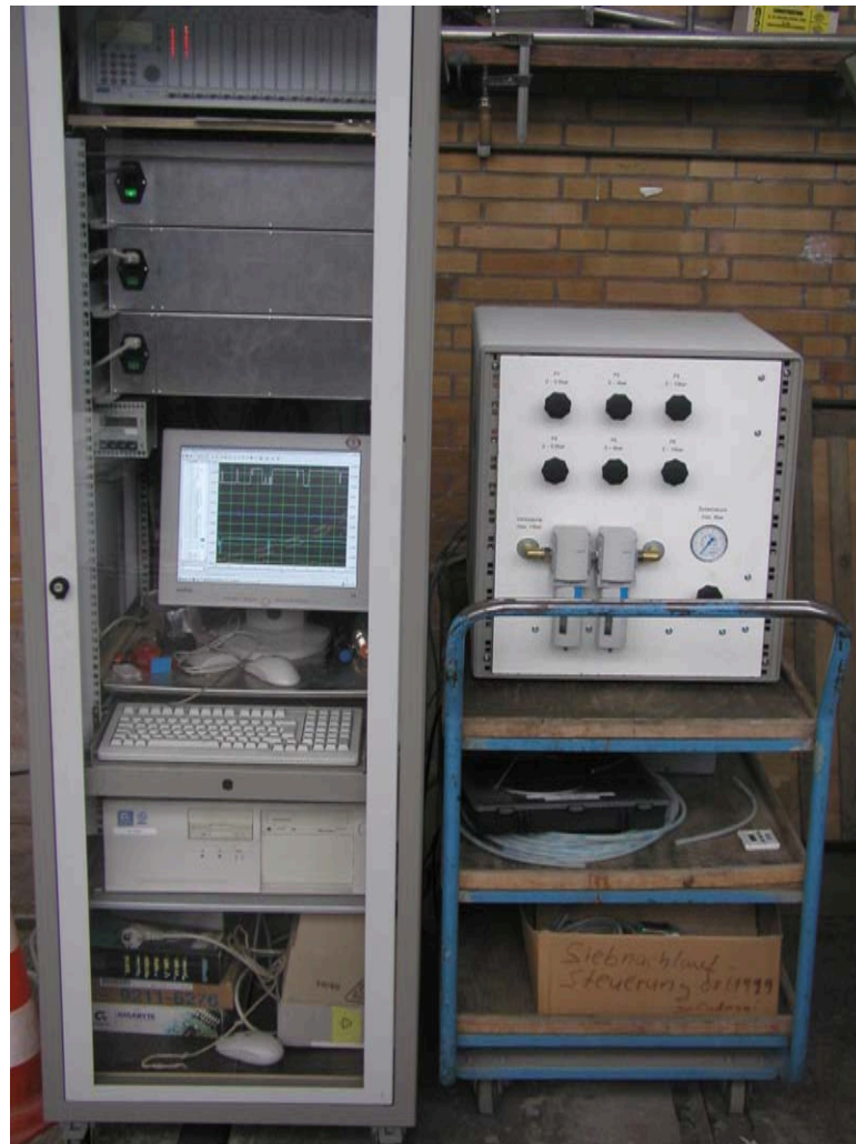
Figure B.1.: Control and measurement equipment: pneumatic unit at the right side, PC and data-locker on the left site.
