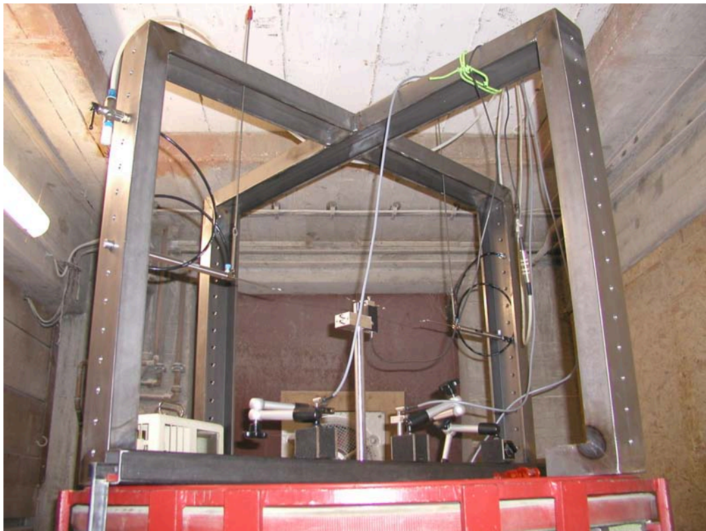
(b) View on the loading frame on top of the former triaxial cell
