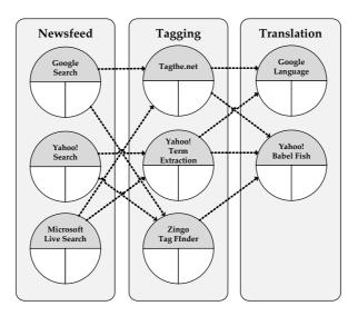
Figure 2.16: Blueprint of a translation and tagging service mashup.
