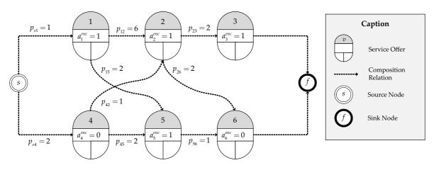
**Figure 3.13:** Service value network with service offers exposing memory-dependent attribute types.
