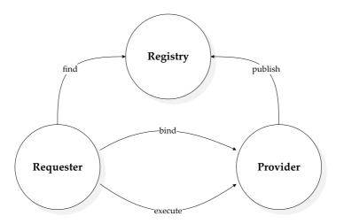
Figure 2.7: Roles and primary operations in service-oriented architectures.
