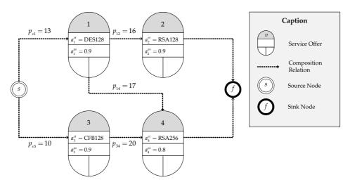
Figure 4.3: Service value network with semantic QoS characteristics.
