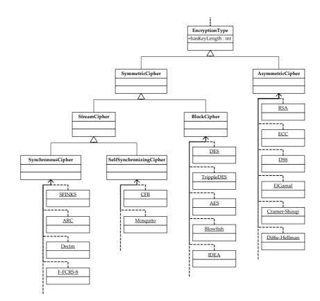
Figure 4.4: Security encryption ontology.
