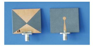
Figure 5.9: The investigated Bow-tie antenna: front side (left) and rear side (right).
