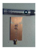
Figure 4.2: The fabricated antenna with the integrated bandpass filter.
