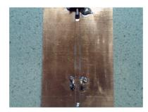
Figure 6.12: Fabricated shaping filter for the Bow-tie antenna.
