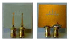
**Figure 3.20:** The fabricated filter with integrated lowpass-highpass sections: rear side (left) and front side (right).
