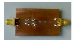
Figure 3.25: The realized CPW filter structure.
