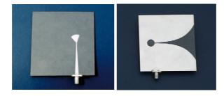
Figure 5.7: The investigated Vivaldi antenna: rear side (left) and front side (right).
