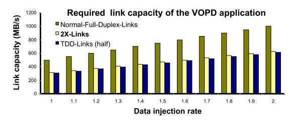
Figure 9.14: Appropriate link capacity of the VOPD application
