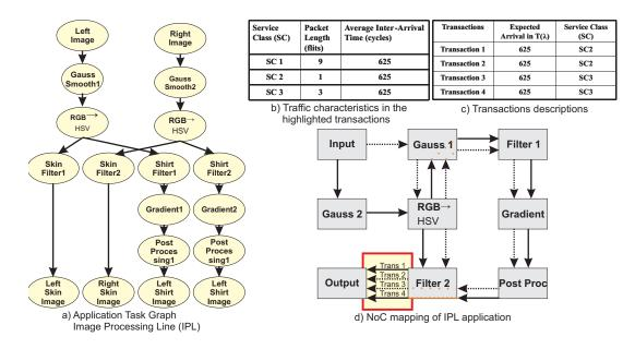
Figure 4.10: IPL mapping and VCBs reduction through probabilistic analysis
