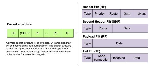
Figure 3.2: Flit composition of a packet for the application-specific NoC
