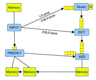
Figure 3.9: MPEG4 video decoder and its data flow graph
