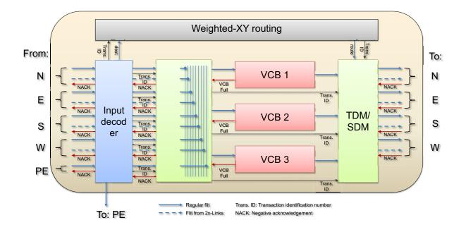
Figure 7.9: An overview of the AdNoC architecture-level part in each router
