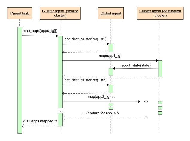
Figure 6.3: Cluster negotiation and application mapping inside the negotiated cluster
