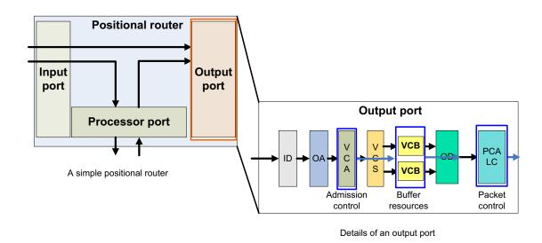
Figure 3.4: The basic QoS-supported router architecture
