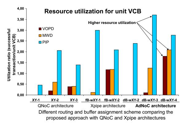
Figure 9.10: Resource utilization for unit virtual channel buffer block
