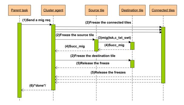
Figure 6.5: Task migration to support runtime application mapping
