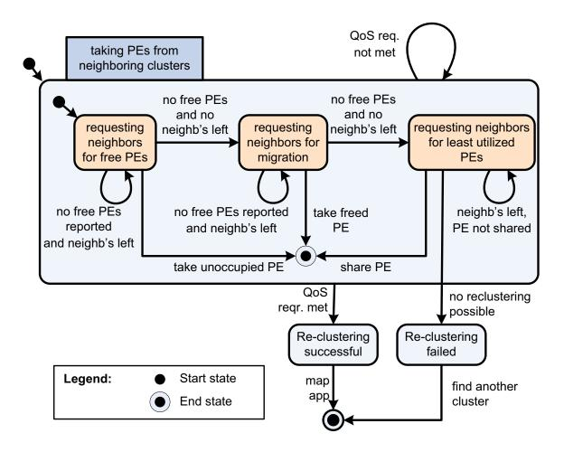
Figure 6.6: The (re-)clustering algorithm flow
