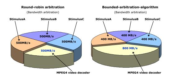
Figure 3.11: Transaction-specific bandwidth provides the lower bound guarantee
