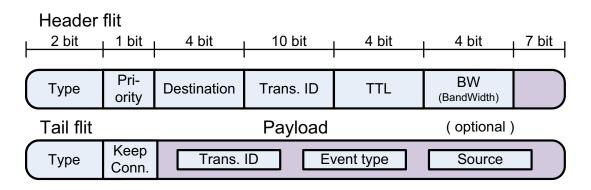
Figure 7.8: Flit composition of a monitoring packet
