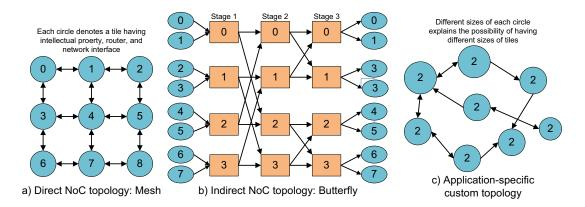
Figure 4.2: Different types of topology for the application-specific NoC design
