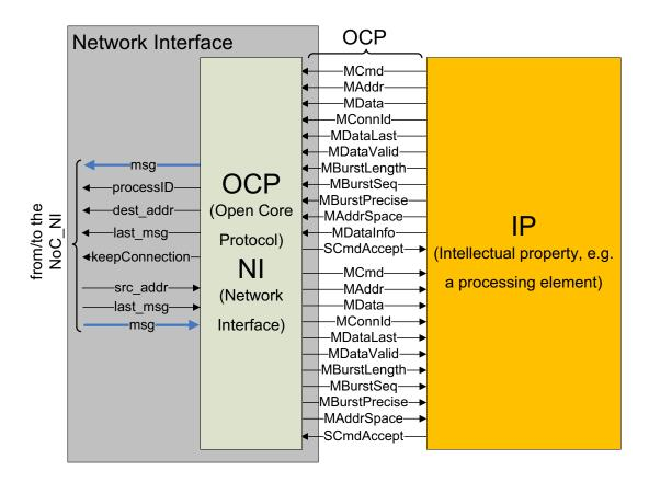
Figure 8.5: An overview of the OCP implementation with its signals
