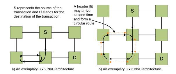
Figure 7.4: Examples of circular routing from the source S to the destination D
