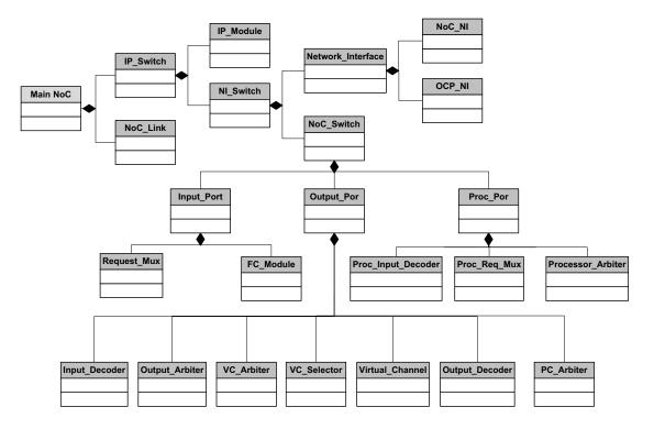
Figure 8.4: The class structure of the configurable NoC (a library structure)
