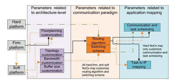
Figure 4.4: Design flow for an application-specific NoC motivated from [122]
