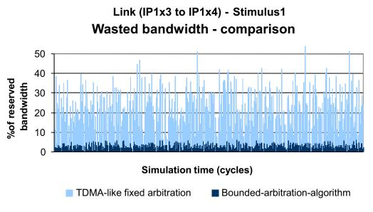
Figure 3.14: Resource utilization: TDMA-like fixed and BAA
