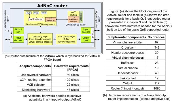
(b) Hardware requirements of a 4-input/4-output router implementation (without adaptive part)
