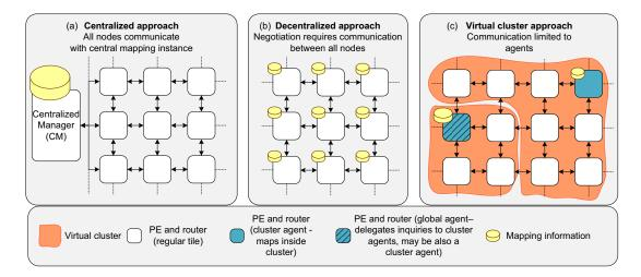
Figure 6.1: Various options for (re-)mapping
