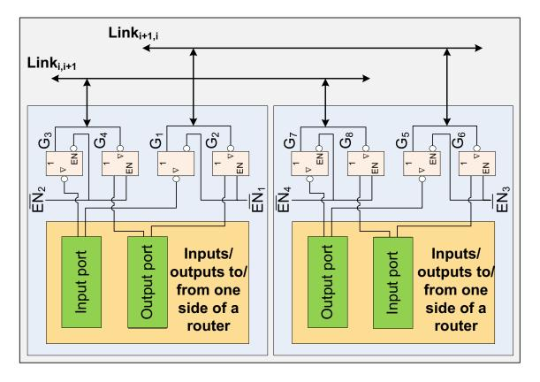
Figure 7.11: Hardware implementation of the 2X-Link
