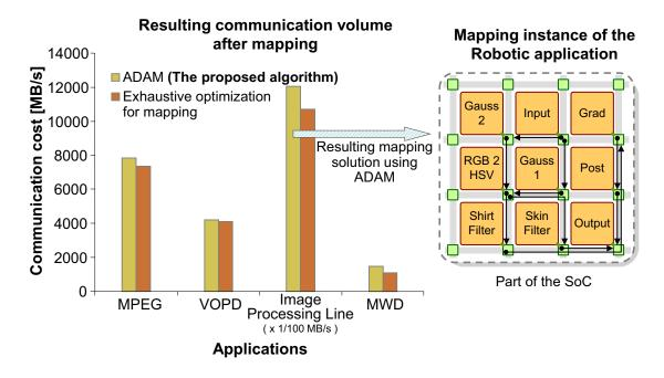
Figure 9.8: Comparing ADAM algorithm to exhaustive offline mapping algorithm
