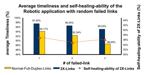
Figure 9.15: Average timeliness and fault-tolerance ability of the Robotic application
