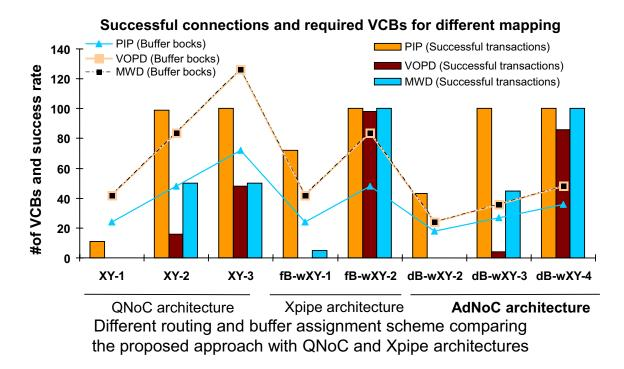
Figure 9.9: Successful transactions and corresponding buffer requirement
