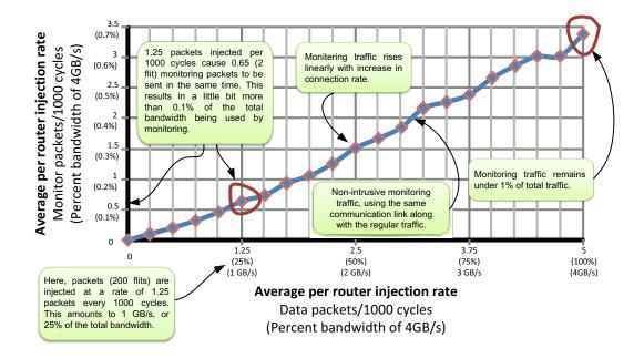
Figure 9.17: Monitoring packets injection and traffic density
