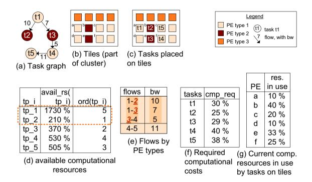
Figure 6.7: Example for a runtime application mapping inside a cluster
