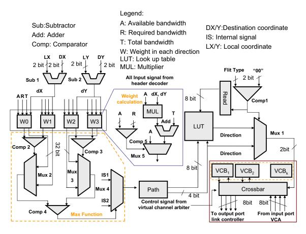
Figure 7.10: Adaptive hardware for the output port of a router
