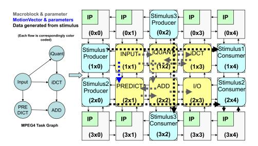
Figure 3.10: MPEG4 video decoder mapping onto a  $5 \times 4$  Mesh
