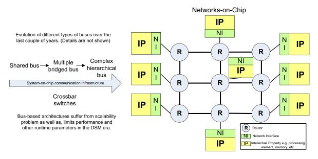
Figure 1.1: Evolution of the Networks-on-Chip
