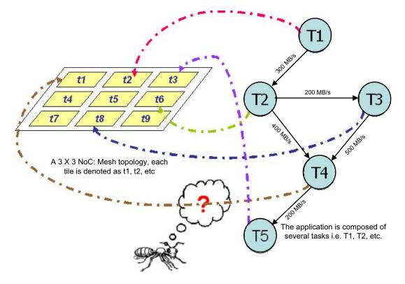
Figure 4.8: Exemplary application mapping onto a 3 x 3 NoC using ACO
