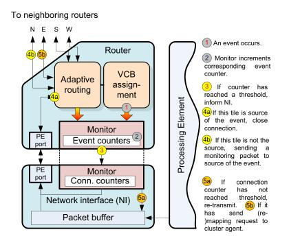
Figure 7.6: Overview of the monitoring component
