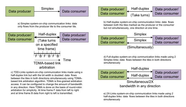
Figure 7.3: Different types of system-on-chip communication links
