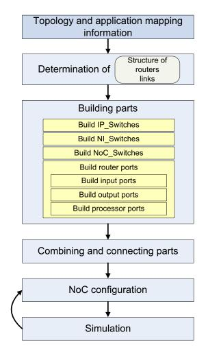
Figure 8.6: Design flow of the NoC architectures having different dimensions
