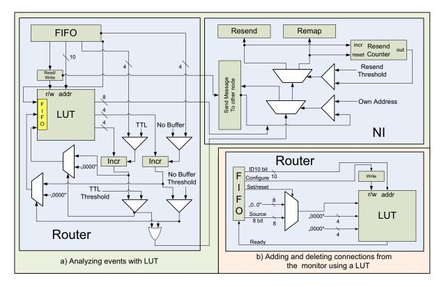
Figure 7.13: Hardware for adding and analyzing monitoring events
