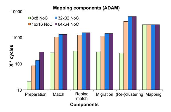
Figure 9.5: Computation complexity of the components of the ADAM algorithm
