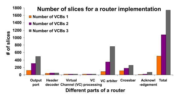
Figure 4.3: Area effects of the increasing virtual channel buffers
