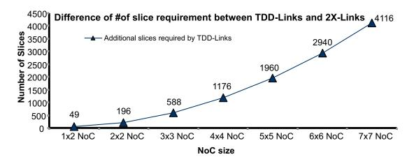
Figure 7.12: Overhead of the TDD-Links compared to the 2X-Links
