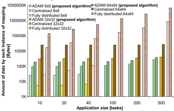
Traffic produced to collect the current MPSoC state
