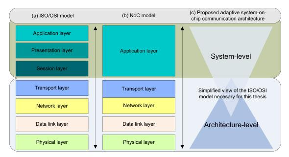
Figure 3.1: Adaptation of the ISO/OSI reference model
