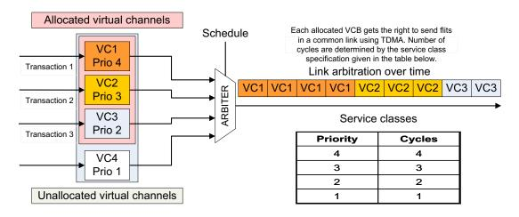
Figure 3.7: TDMA: Time division multiple access-like link arbitration
