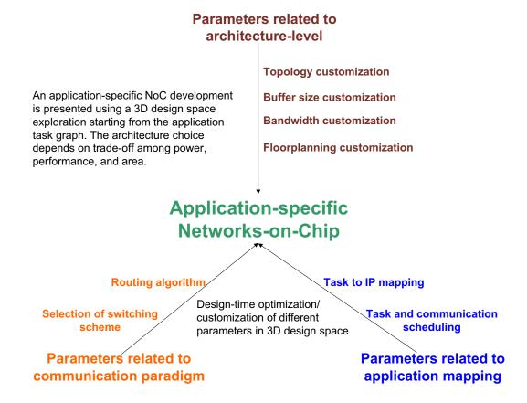
Figure 4.1: 3D design-space exploration for the application-specific NoC design
