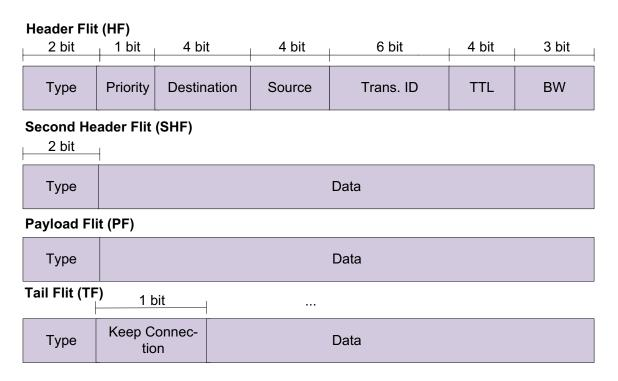
Figure 3.3: Exemplary flit composition of a 4 x 4 adaptive NoC
