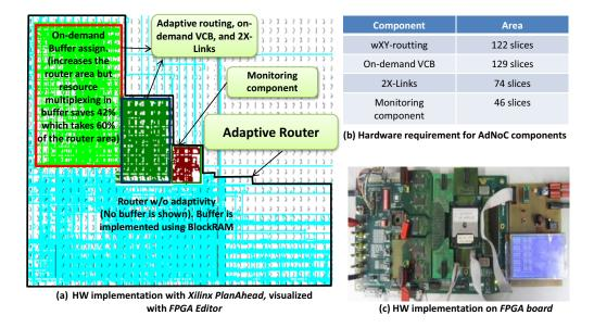
Figure 8.7: Hardware prototyping of the NoC architectures
