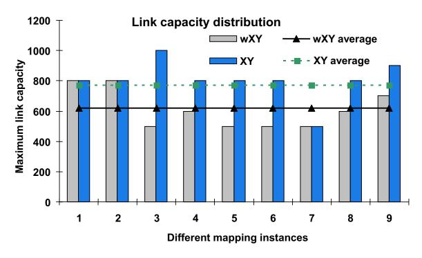
Figure 9.11: Utilization of the link capacity (VOPD application)
