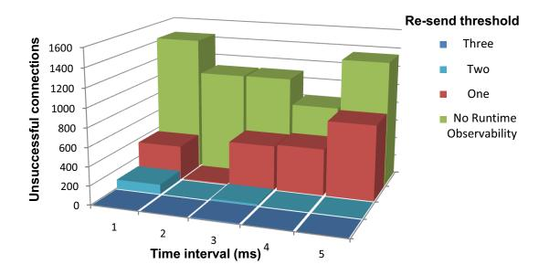
Figure 9.19: Unsuccessful transactions for various re-sending thresholds
