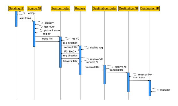
Figure 3.5: Example of a packet transmission and requesting directions
