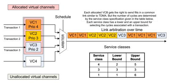
Figure 3.8: Proposed bounded-arbitration-algorithm
