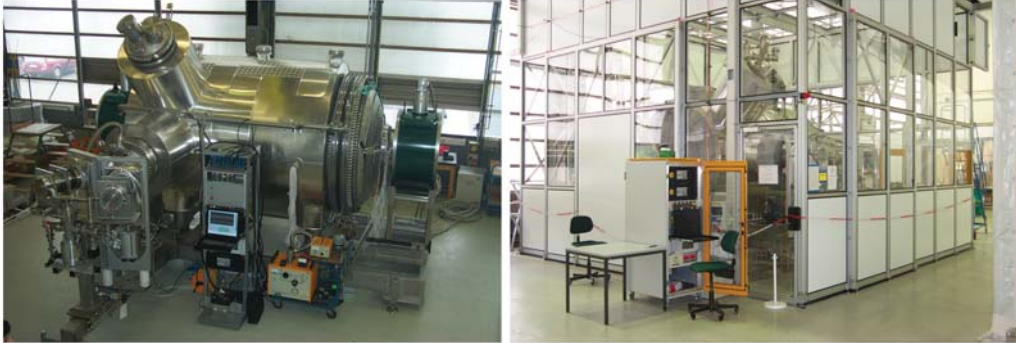
Figure 3.2: Pre-spectrometer setup without satellite systems of detector and e-gun. The left picture shows the pre-spectrometer vessel with the cylindrical main body already equipped with thermal insulation. Attached to the horizontal pump port is the pump system. Magnets are in place to the left and right of the vessel. Right picture: dry air cabin enclosing the spectrometer vessel. The dry air cabin has two functions, a) prevention of air exchange to allow dehumidifying of air to lower the dew point, b) access restriction during high voltage operation.
