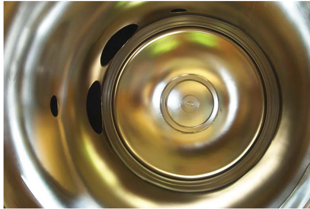
Figure 3.5: Electropolished inner surface of the pre-spectrometer. During the electropolishing process the surface is deburred, effectively reducing the surface area and improving high voltage stability as well as cleanliness performance. Visible are the openings to the two pump ports, the western chimney and the side-port.
