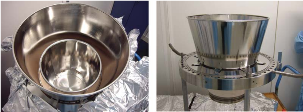
Figure 4.12: Picture showing the novel Anti-Penning electrode (APE) and stainless steel earth electrode mounted together onto the DN500 flange with conical isolator. The APE is attached with screws to the inside of the DN500 flange, the earth electrode is fixed to the DN200 flange of the conical insulator.
