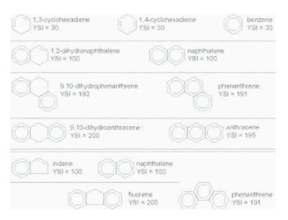
Figure 2. Sooting tendencies and molecular structures of several aromatic hydrocarbons containing cyclohexadienyl, cyclopentadienyl, and benzenoid rings.
