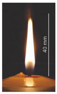
Figure 1. Color image of a candelilla candle flame at its smoke point. This smoke point is 37.0 mm, the wick diameter is 1.7 mm, and the and wick length is 9.3 mm. These dimensions are slightly different from the mean values reported elsewhere in this manuscript.
