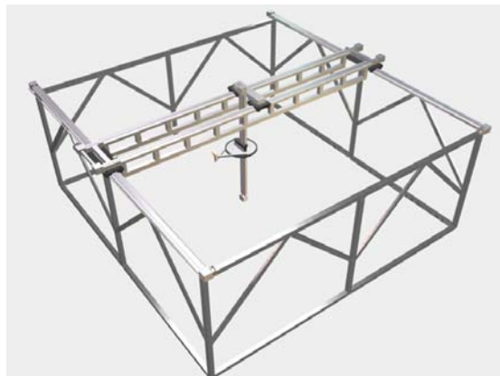
Figure 4: An impression of the complete setup with portal carrier and parallel SCARA manipulator.
