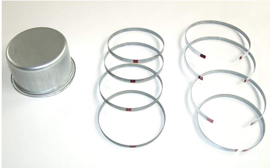
Figure 2: Springback experiment: cup, rings, open rings
