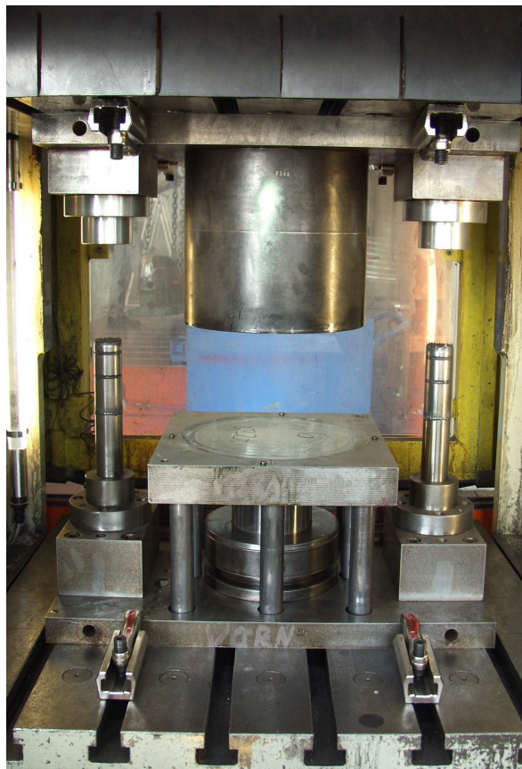
Figure 1: Cup drawing tool setup
