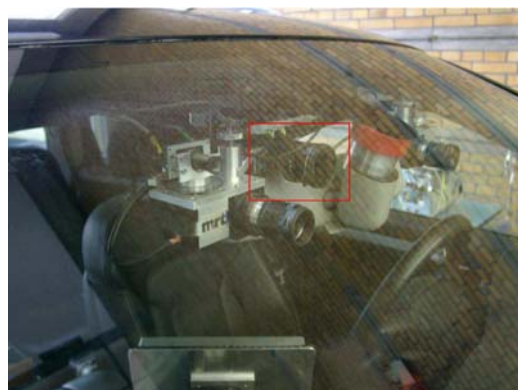
Figure 2 - Dedicated camera platform mounted behind front window. [3]
