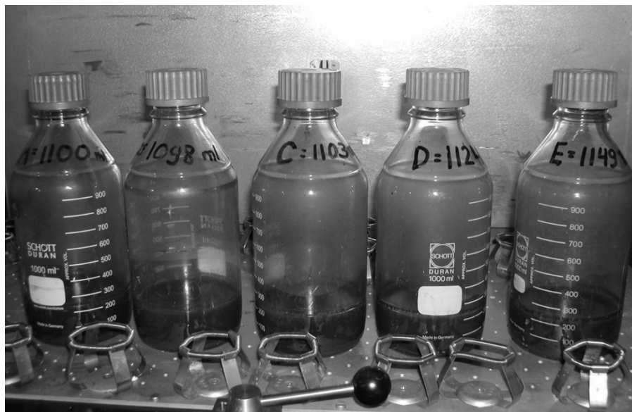
Figure 3.7 Batch assays using Schott bottles for determination of the methane production potential of press water and potato sludge
