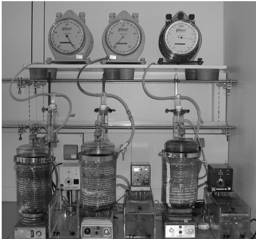
Figure 3.6 Reactor set-ups for determination of the biogas production potential of biowaste and foodwaste experiment
