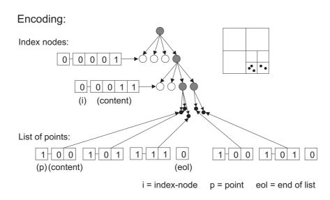
Figure 4.10: Encoding of a quadtree
