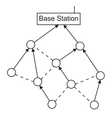
Figure 2.2: Routing tree as an overlay over the connectivity graph of the network
