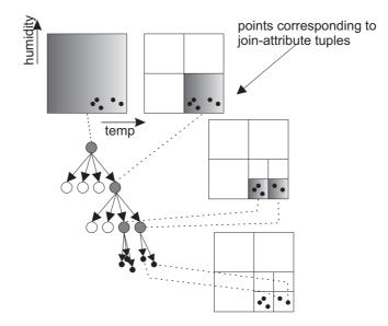
Figure 4.9: Construction of the quadtree
