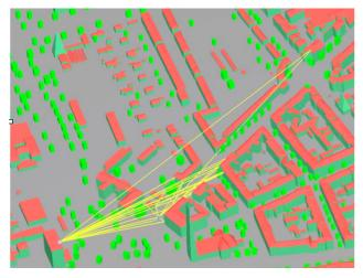
Fig. 5 Ray-tracing in a virtual scenario, here C2 base station
