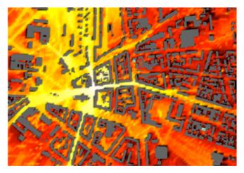
Fig. 3 Typical coverage prediction for 3G communications
