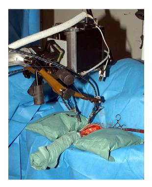
Figure 3.5: Experimental setup for osteotomy of an exposed sheep tibia using the  $CO_2$  laser osteotome. (With kind permission from Springer Science+Business Media: [Kut10])
