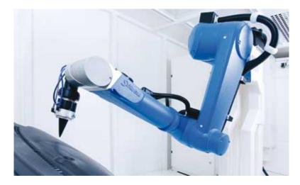
Figure 2.8: Next generation of robot-based CO<sub>2</sub> laser systems Votan C-BIM (Beam in Motion) with incorporated optical path. (Picture: JENOPTIK Automatisierungstechnik GmbH.)
