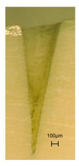
Figure 4.27: Microscopic image of an exemplary wobble cut profile after 80 consecutive lines with focal position at the surface at 40 µs pulse duration,  $r_{wobble} = 200 \,\mu\text{m}$ ,  $v_l = 40 \,\text{mm/sec}$ ,  $f_{laser} = 200 \,\text{Hz}$  and  $f_{wobble} = 135 \,\text{Hz}$ . The cutting depth is 1896.73 µm and width 609.54 µm.
