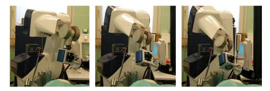
Figure 7.4: For processing the predefined line marking path the robot positions the scan head relative to the skull in the three optimized locations. Compare Figure 7.3.
