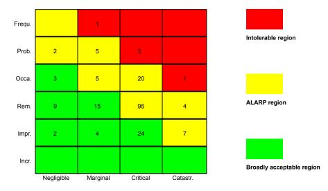
Figure A.8: All risks of the system for robot assisted laser osteotomy assigned to the risk graph according to their severity.
