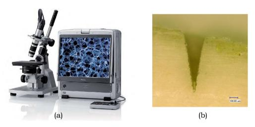
Figure 4.4: Digital microscope (VHX-600, Keyence Corp., Osaka, Japan) and an exemplary microscopic view on a cutting profile of bony specimen.
