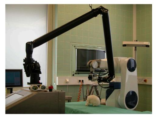
Figure 6.6: The experimental setup for robot assisted laser osteotomy.
