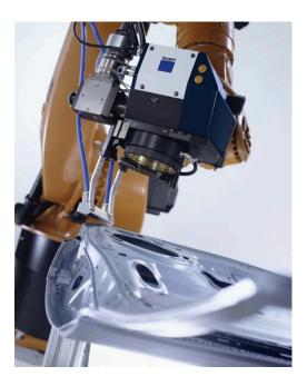
Figure 2.9: Remote laser welding with a robot positioning a threedimensional scanning device relative to a workpiece. (Picture: TRUMPF GmbH + Co. KG.)
