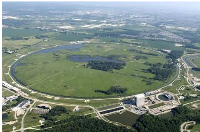
Figure 2.1: Aerial view of the Tevatron collider at the Fermilab site. The circular ring is the Tevatron maintenance road, the collider itself is located in a tunnel eight meters below the surface. At the eight o'clock position the CDF site is located, while DØ sits at the twelve o'clock position.
