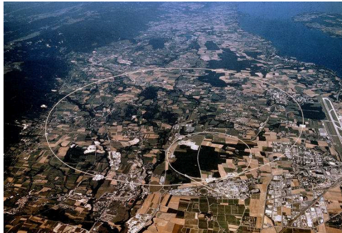
Figure 2.4: Aerial view of the CERN site near Geneva located at the five o'clock position of the main ring. The white lines indicate the location of the several preaccelerators and the LHC below the surface.
