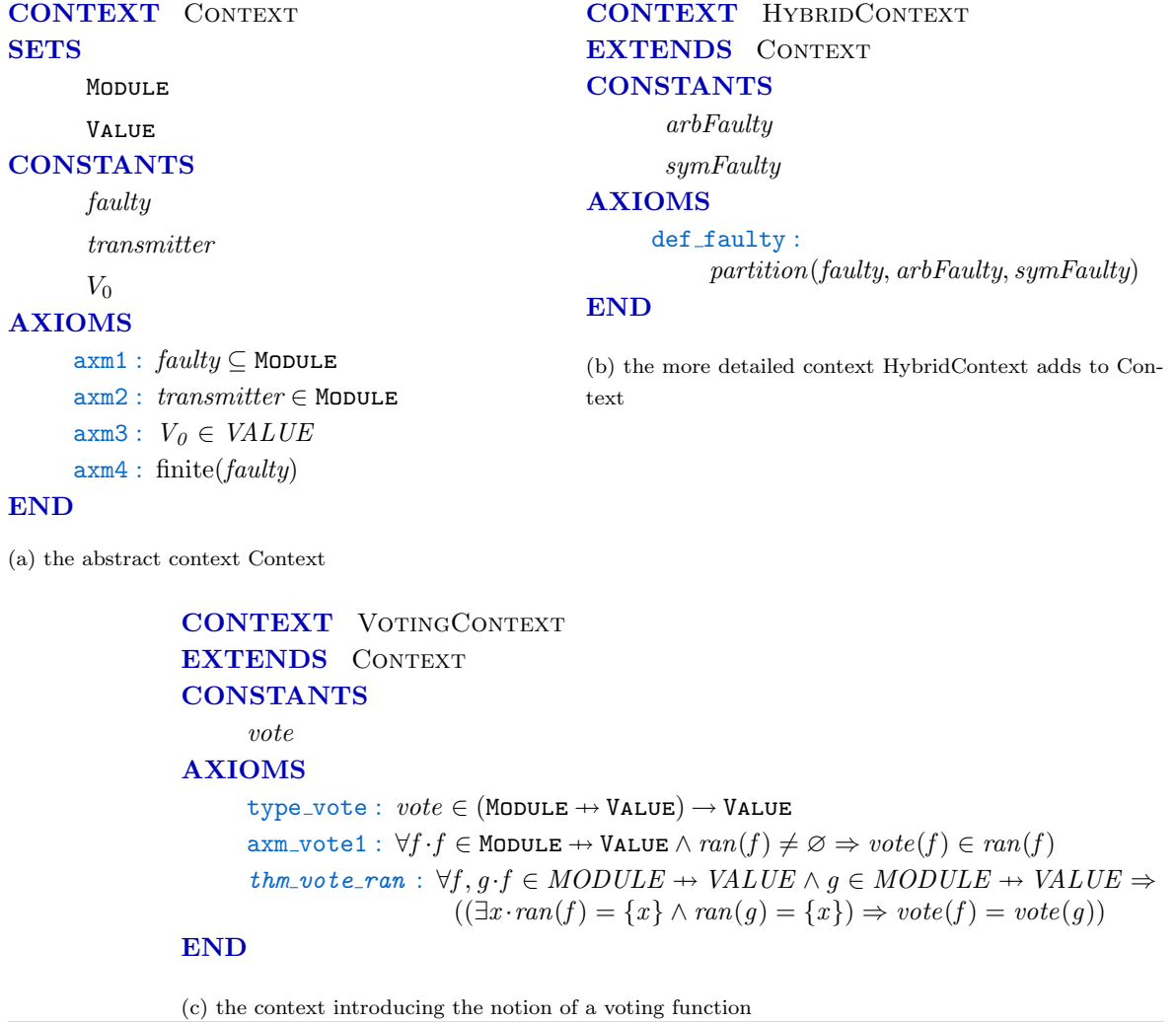
Figure 3: Contexts used by the machines in the model
