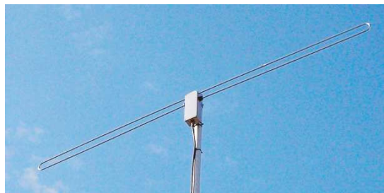
Figure 4.3: The beacon dipole antenna used used to monitor the timing from LOPES
