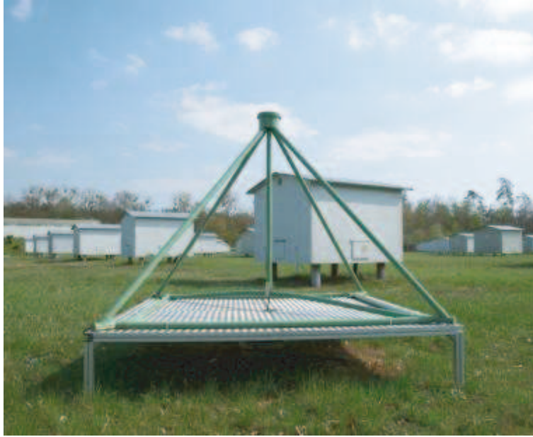
Figure 4.1: A LOPES antenna at the site within the field of the particle detector array KASCADE-Grande.
