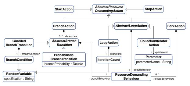
Figure 2. RDSEFF control flow primitives (from [5])
