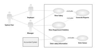
Fig. 2. The salary viewing system, Use Case diagram
