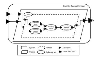
Fig. 3. Stability Control System Mapped in AADL
