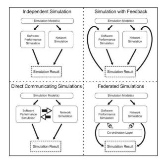
Fig. 3. Coupling of software and network simulations
