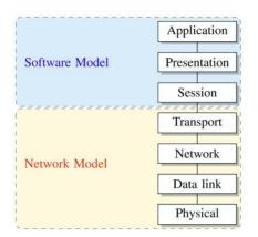
Fig. 1. OSI stack with the network model and the software model.
