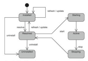
Fig. 2: The lifecycle of an OSGi component [1].
