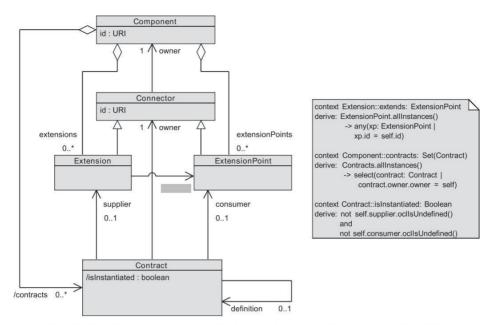
Fig. 1: The Treaty meta model (derived fields are defined using OCL [22]).
