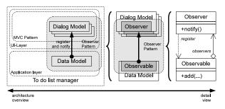
Fig. 2: Refinement of a usage relationship
