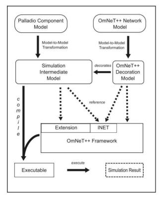
Fig. 4. Schematic illustration of our integrated simulation approach
