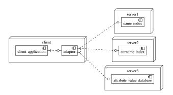
Fig. 11. Structural and deployment view of our separated CRM database. The indices are deployed on separate servers as well as the encrypted attribute values database. An adaptor deployed on the clients' machine provides a standard SQL interface to the client application. The overall service consists of the indices, the adaptor and the attribute values database.
