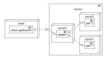
Fig. 5. System and deployment view of a parallel separation of a service, and an adaptor. The composition structure and the deployment relationship may cross each other. Consider the adaptor deployed on the client. This is not in conflict with UML and conceptionally sound, as long as the inner components are bundled by an *assembly* where inner components remain visible, exactly for the reason of possibly distributed deployment.
