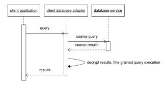
Fig. 4. Sequence Diagram for a query in the serial separated database. The adaptor translates queries from the client application to match the scheme of the encrypted database of the database service decrypts the results and returns them after removing false positives to the client application.
