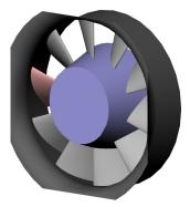
Figure 4.6: Simplified Geometry: Blower Assembly
