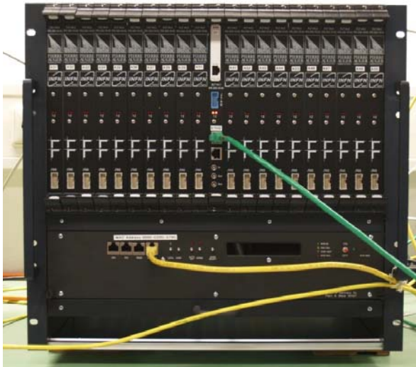
Figure 2. Image of the DAQ system in the USCT configuration. It is composed of one Second Level Card (SLC) for measurement control and communication management (middle slot) and 20 First Level Cards (FLC) for parallel sensor signal acquisition and data storage.
