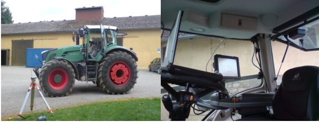
Fig. 1 Fendt 936 Vario tractor and its cabin with machine guidance terminal
