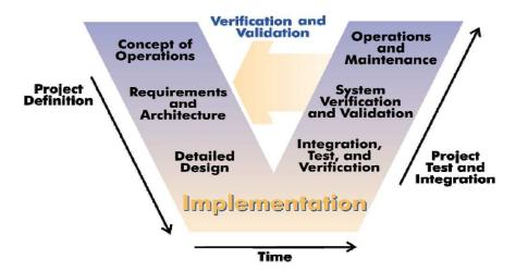
Fig. 2.2. V-Model Process Visualization (Source: Osborne et al., 2005, p. 20)
