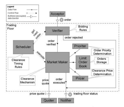
Fig. 2.12. Detailed view on GEM's "trading floor" component (Source: Rachlevsky-Reich et al., 1999)
