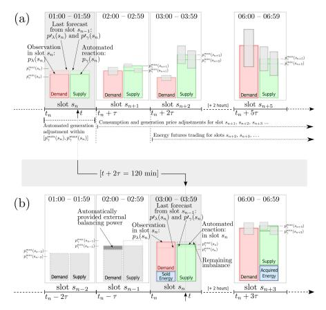
Fig. 5.10. Broker's expected and actual energy supply and demand at two points in time.
