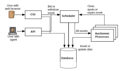
Fig. 2.11. Schema of AuctionBot's System Architecture (Source: Wurman et al., 1999)
