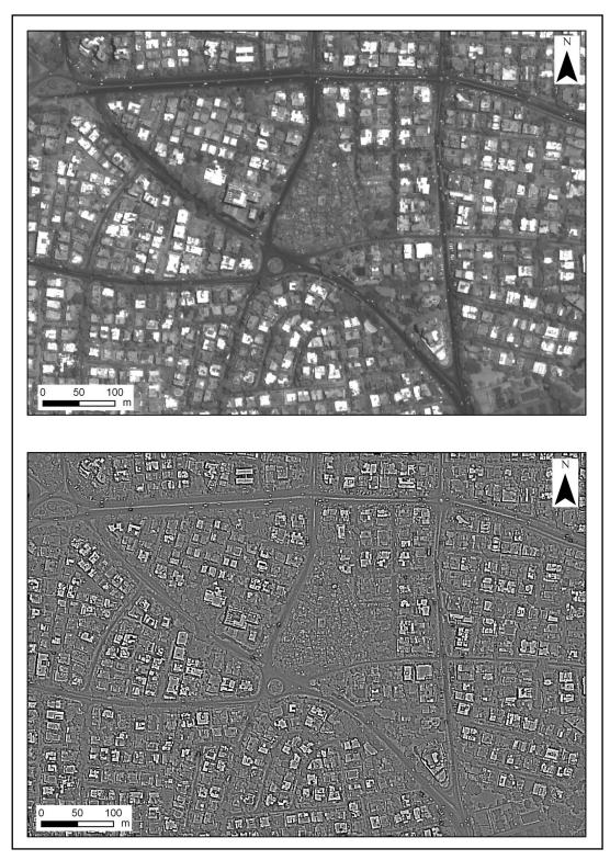
Figure 35: High pass filter with a kernel size of 3 applied to the panchromatic Quickbird image.
