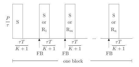
Figure 6.11: Transmission model for BAF with incremental relaying and an arbitrary number of relay nodes.  $R_m$ ,  $m \in \{1,2\}$ , and  $R_n$ ,  $n \in \{1,2,\ldots,K\}$ , describe the transmitting relay depending on prior transmissions.
