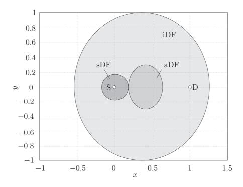
Figure 6.6: Regions in which  $\epsilon$ -outage capacity of the cooperative relaying protocols outperforms  $\epsilon$ -outage capacity of transmit diversity for  $\epsilon = 10^{-4}$ , SNR = 20 dB, and  $\alpha = 3$ .
