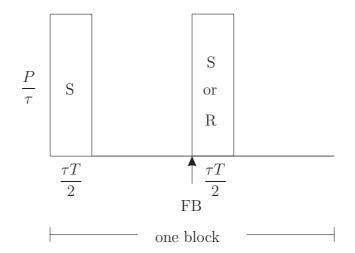
Figure 6.8: Transmission model for incremental relaying with AF and BAF. If the source transmission succeeded (feedback FB = 1), the source transmits during the second sub-block, too. If the source transmission failed (feedback FB = 0), the relay aids communication during the second sub-block.
