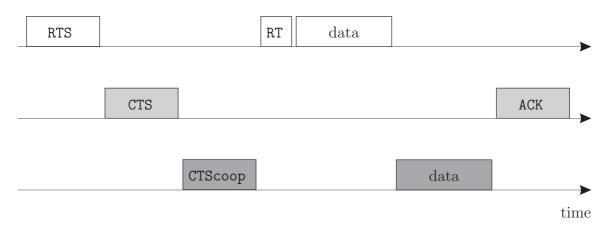
*Figure 3.3:* General functionality of the adaptive relay selection protocol (ARSP), where one relay has been selected.
