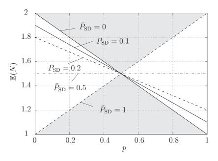
Figure 6.13: Average amount of required sub-blocks  $\mathbb{E}(N)$  vs. reliability p of the feedback channel for the one-relay case.
