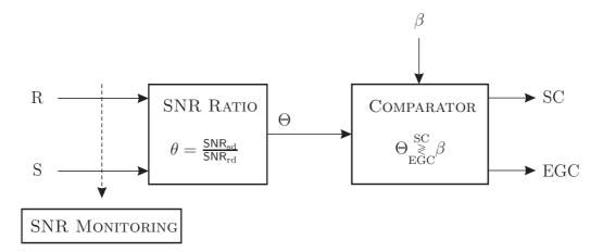
*Figure 5.3:* Structure of a dual-diversity combining receiver that selects between selection combining (SC) and equal gain combining (EGC) on the basis of an SNR criterion.
