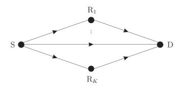
Figure 2.4: Principle of a multi-route network with one source S, K relays  $R_k$ ,  $k = 1, \ldots, K$ , and one destination D.
