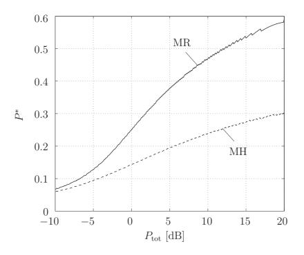
Figure 4.7: Optimal power allocation  $P^* = \tau^* P_{\rm s}/P_{\rm tot}$  for the source. The distance source-relay has been set to  $d_{\rm sr} = 0.3$ .
