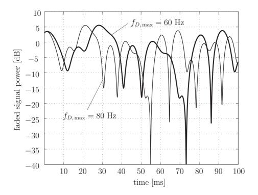
Figure 1.1: Faded signal power [dB] of a signal that is transmitted over two different Rayleigh fading channels with a maximum Doppler shift of  $f_{D, \max} = 80$ Hz (thin line) and  $f_{D, \max} = 60$  Hz (thick line), respectively. Sampling time equals 100  $\mu$ s.
