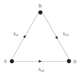
Figure 5.1: Statistically symmetric relay network with source S, relay R, and destination D. Statistically symmetric means that in average all channel coefficients are equal.
