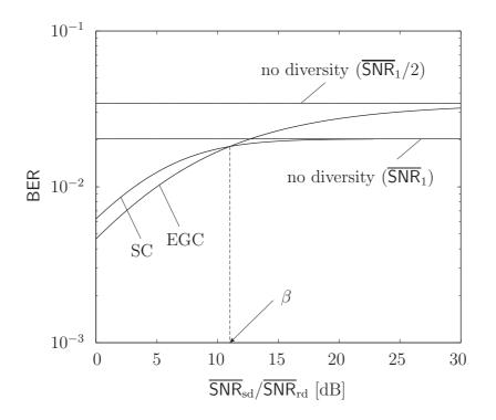
Figure 5.4: Bit error rate (BER) of selection combining (SC) and equal gain combining (EGC) for BPSK with respect to branch unbalance  $\overline{\mathsf{SNR}}_{sd}/\overline{\mathsf{SNR}}_{rd}$  [dB]. Parameter  $\overline{\mathsf{SNR}}_{sd}$  was set to 5 dB.
