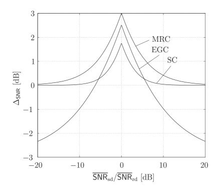
Figure 5.2: Comparison of the SNR gain  $\Delta_{SNR}$  of selection combining (SC), equal gain combining (EGC), and maximal ratio combining (MRC) with respect to branch unbalance  $\overline{SNR}_{sd}/\overline{SNR}_{rd}$  [dB].
