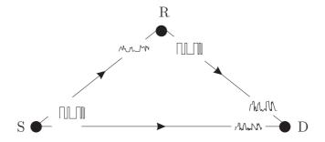
Figure 2.8: The functionality of decode-and-forward (DF).
