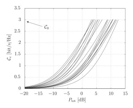
Figure 4.10: Delay-limited capacity vs. total transmit power for selective multi-route and the parameters  $d_{\rm sr} = 0.2$  and  $\alpha = 4$ .
