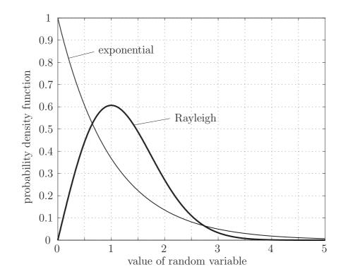
Figure 2.2: Probability density function of a Rayleigh and exponential random variable for  $\sigma^2 = 1$ , respectively. For the Rayleigh distribution the random variable is |h|, and for the exponential distribution the random variable is  $|h|^2$ .
