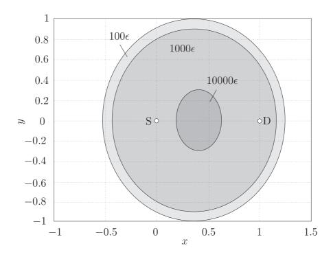
Figure 6.7: Regions where  $\epsilon$ -outage capacity of incremental relaying with decode-andforward outperforms  $\epsilon$ -outage capacity of transmit diversity for different values of Pr("source transmission fails") as a function of  $\epsilon$ . Parameters are  $\epsilon = 10^{-4}$ , SNR = 20 dB, and  $\alpha = 3$ .
