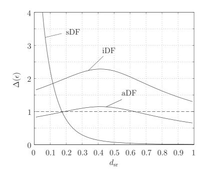
Figure 6.5: Ratio between  $\epsilon$ -outage capacity of relaying protocols and transmit diversity vs. source-relay distance  $d_{\rm sr}$  for  $\epsilon = 10^{-4}$ , SNR = 20 dB, and  $\alpha = 3$ . Curve sections that are above the dashed line indicate regions in which the cooperative protocols outperform transmit diversity.
