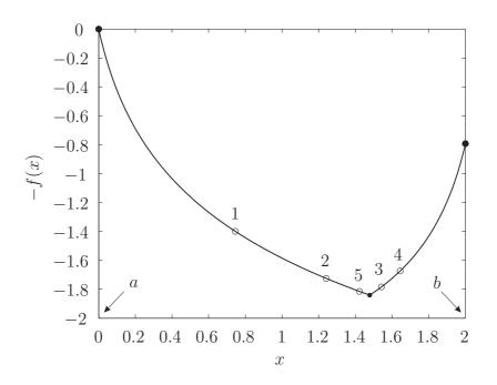
Figure 4.5: Operating mode and the first five iteration steps of the optimization algorithm on the interval [a,b] = [0,2]. Point 1 is the initial value. Points 2 and 3 have been found by golden section search, whereas points 4 and 5 have been found by parabolic interpolation (cf. Tab. 4.1).
