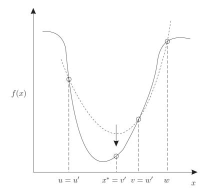
Figure 4.4: Parabolic interpolation.
