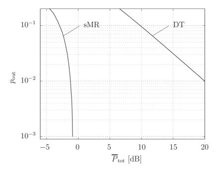
Figure 4.14: Outage probability of selective multi-route and direct transmission vs. averaged total transmit power for  $C_0 = 1$  bit/s/Hz,  $d_{\rm sr} = 0.2$ , and  $\alpha = 4$ .
