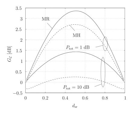
Figure 4.9: Capacity gain  $G_{\mathcal{C}}$  of multi-route and multi-hop over direct transmission when optimized power allocation  $P^*$  and optimized time allocation  $\tau^*$  are used.
