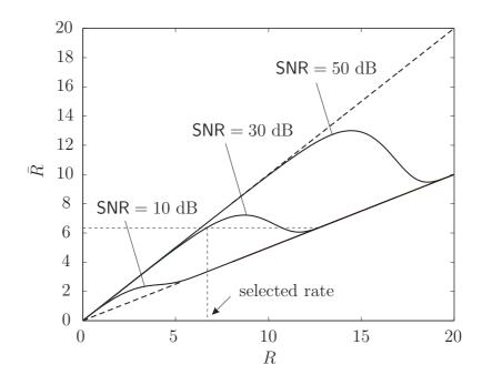
Figure 6.1: Mapping of R to  $\overline{R}$ . Dashed lines illustrate upper and lower bounds. The upper bound is given by  $\overline{R} = R$  and the lower bound is given by  $\overline{R} = R/2$ . In [37] the smallest R out of those is selected that determine the same  $\overline{R}$ .
