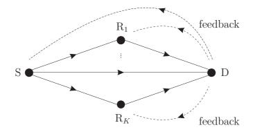
Figure 2.6: Principle of an incremental relaying network with one source S, K relays  $R_k, k = 1, ..., K$ , and one destination D.
