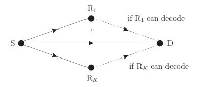
Figure 2.5: Principle of an adaptive multi-route network with one source S, K relays  $R_k, k = 1, ..., K$ , and one destination D.
