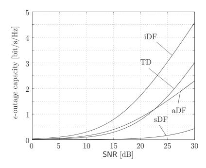
Figure 6.4:  $\epsilon$ -outage capacity in bit/s/Hz vs. SNR in dB for an outage probability of  $\epsilon = 10^{-4}$  and  $\alpha = 3$ . The relay has been placed at  $d_{\rm sr} = 0.5$ .
