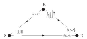
Figure 2.7: The functionality of amplify-and-forward (AF).
