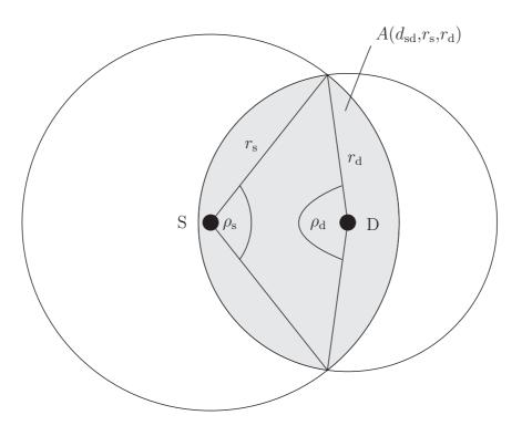
Figure 3.1: Relay area  $A(d_{\rm sd}, r_{\rm s}, r_{\rm d})$ .
