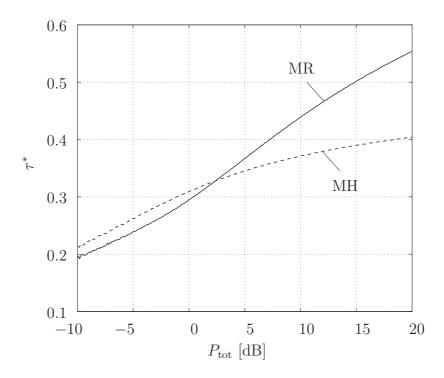
Figure 4.8: Optimal time allocation  $\tau^*$  for the source. The distance source-relay has been set to  $d_{\rm sr} = 0.3$ .
