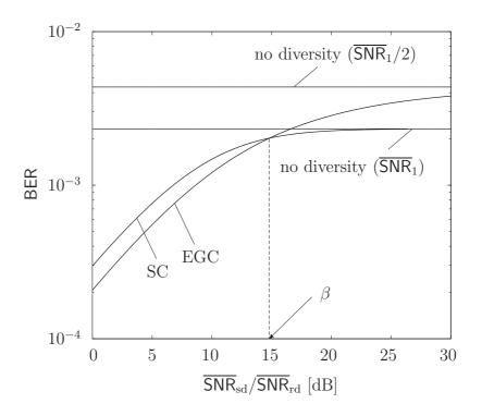
Figure 5.5: Bit error rate (BER) of selection combining (SC) and equal gain combining (EGC) for BPSK with respect to branch unbalance  $\overline{\mathsf{SNR}}_{sd}/\overline{\mathsf{SNR}}_{rd}$  [dB]. Parameter  $\overline{\mathsf{SNR}}_{sd}$  was set to 10 dB.
