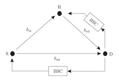
*Figure 6.12:* Network for incremental relaying with imperfect feedback modeled as binary symmetric channel (BSC).
