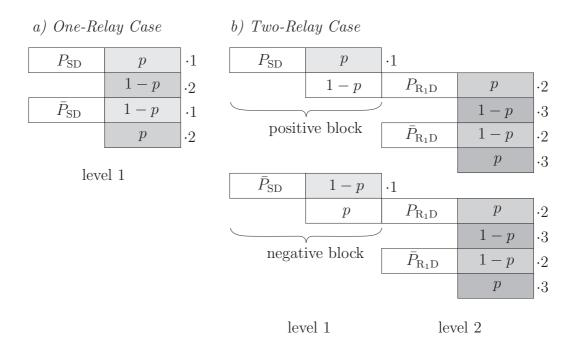
Figure 6.16: Binary tree-based construction in order to calculate the average amount of required sub-blocks  $\mathbb{E}_K(N)$ . a) One-relay case and b) two-relay case. Number of levels corresponds to the number of relays in the network.
