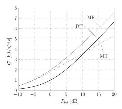
Figure 4.6: Instantaneous channel capacities with optimal resource allocation for multi-hop (MH) and multi-route (MR) in bit/s/Hz. The distance source-relay has been set to  $d_{\rm sr} = 0.3$ . Capacity of direct transmission (DT) is illustrated as reference.
