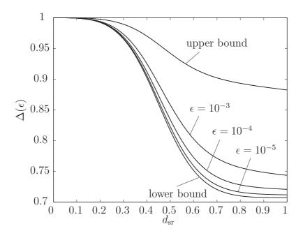
Figure 6.9: Ratio  $\Delta(\epsilon)$  of the  $\epsilon$ -outage capacity of incremental relaying with decodeand-forward to the cut-set bound for  $g \to 0$  and  $\alpha = 3$ .
