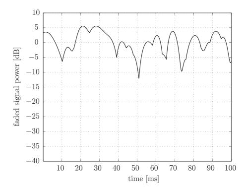
Figure 1.2: Faded signal power [dB] of a signal that is transmitted over the two Rayleigh fading channels shown in Fig. 1.1. Only the best among the two paths is selected to demonstrate the benefit of diversity.
