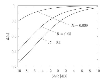
Figure 6.10: Ratio  $\Delta(\epsilon)$  vs. SNR for  $\epsilon = 0.001$  and different values of rate R in bit/s/Hz. The distance source-destination was normalized to 1.
