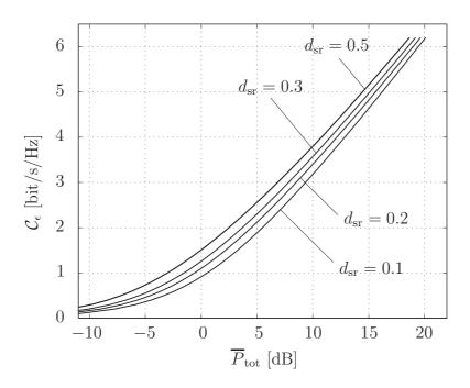
*Figure 4.11:* Delay-limited capacity vs. averaged total transmit power for different relay locations.
