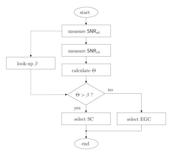
Figure 5.6: Algorithm for the hybrid receiver structure.
