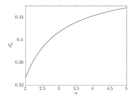
Figure 6.3: Optimal source-relay distance  $d_{\rm sr}^*$  vs. path-loss factor  $\alpha$ . For  $\alpha \to \infty$   $d_{\rm sr}^*$  tends asymptotically to  $d_{\rm sr}^* = 0.5$ .  $d_{\rm sr}^*(\alpha = 2) = 1/3$ .
