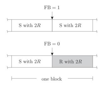
Figure 6.2: Transmission model for incremental relaying. If the source-destination link is not in outage (feedback FB = 1), the source transmits during the second sub-block, too. If the source-destination link is in outage (feedback FB = 0), the relay aids communication during the second sub-block.
