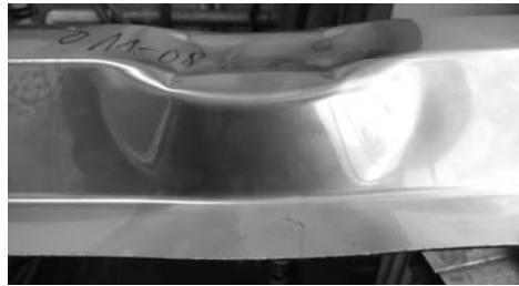
Figure 7: Web crippling failure at intermediate support.
