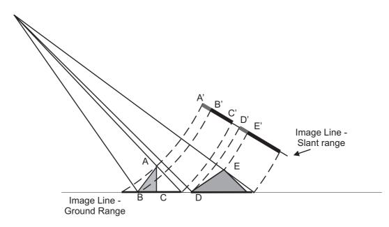
Fig. 7. Image lines in slant- and in ground-range format. Layover effects occurs by steep surfaces. The signal reaches point A before the ground (B). In the image, the signal response from the top is displaced toward the sensor (A'). Radar shadows are present behind steep surfaces or high objects (see C and C'). Tilted surfaces (D-E) appear compressed in slant range(D'-E'), so called foreshortening.
