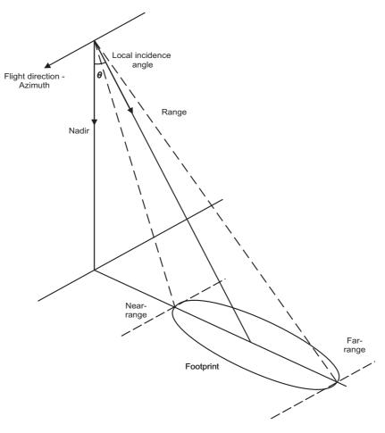
Fig. 6. Side-looking geometry of a SAR-sensor.
