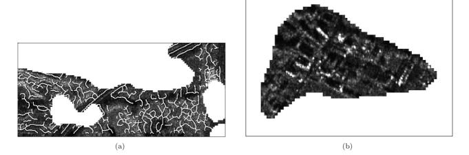
Fig. 45. Global context information is used for suppressing false alarms in forest regions and for concentrating on areas where TUM-LOREX is likely to be successful. (a) Forest regions extracted by a textural classification are highlighted. A line extraction in white show all the extracted line features. Almost all of them are only clutter. (b) Extracted built-up areas are highlighted.
