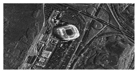
Fig. 11. The football stadium Allianz-Arena can be seen in this TerraSAR-X sub-image. The imaging mode is high-resolution spotlight mode and the data was obtained as radiometrically enhanced data product.
