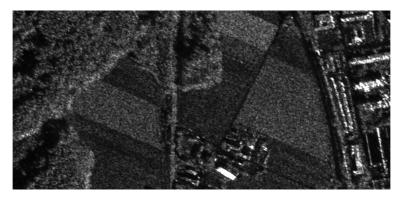
Fig. 9. Strong scattering caused by metallic objects and by double bounce and trihedral bounce reflections can be seen in the left part of the image. This industrial area contain large buildings. The right part show the irregular volume scattering caused by high vegetation.
