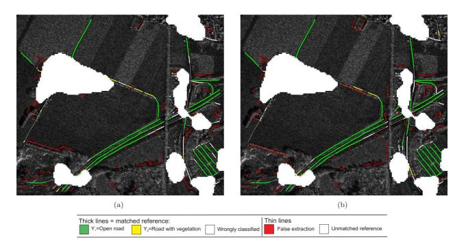
Fig. 53. Results of the dataset Oberpfaffenhofen after fusion  $(BN_3)$ . Input to the fusion are the dark linear features and their uncertainty assessment. Masked built-up areas are white. (a) **Oberpfaffen1-2** shows the fusion of Figs. 52(a) and 52(b) while (b) **Oberpfaffen2-3** shows the fusion of Figs. 52(b) and 52(c).
