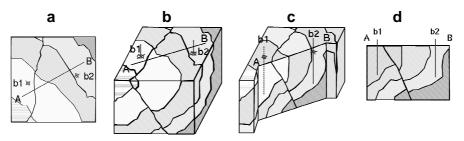
**Figure 1** Example of a 3Dto2D service: Planar profile section between endpoints A and B, with projected borehole profiles b1 and b2. (a) – location in map plane, (b) – block view of 3D model, (c) – view of profile section with part of model removed, (d) – resulting 2D profile section with the projected boreholes.
