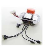
(b) Top view: inertial measurement unit and SSD data storage.
