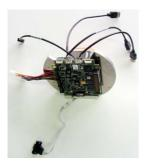
(a) View from below: PCI/104-Module with heat spreader baseplate.
