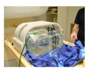
(c) Rear view with closed receive body coil.
