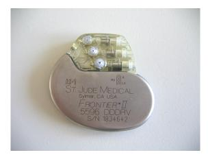
Figure 4.22.: Pacemaker device used for in-vitro test (Frontier II by St. Jude Medical).
