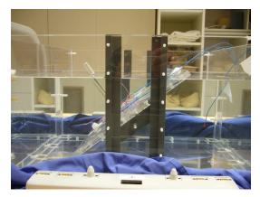
(a) Side view of phantom with object carrier and reference temperature probe in the background.
