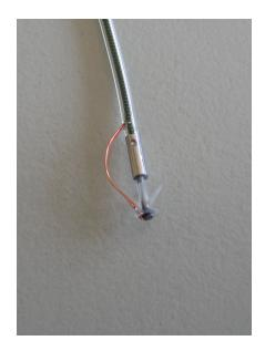
Figure 4.27.: Tip of lead with included thermocouple element and supply line.
