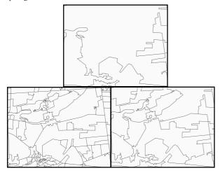
Figure 7. Application example by courtesy of J. Haunert, IKG Hannover University: a section of ca. 2 % of a digital map on land-use at three different scales.
