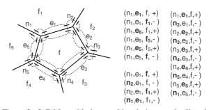
Figure 2. 2-G-Map with darts and involutions, and cell-tuple representation of the orbits around node  $n_1$ , edge  $e_1$  and face f.
