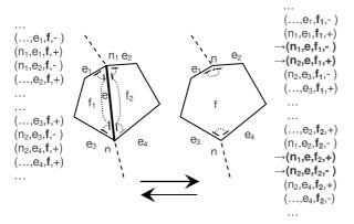
Figure 4. Merging two faces  $f_1$ ,  $f_2$  by removing edge e.
