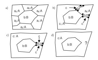
Figure 6. (a) A face *b* of class *B* is completely surrounded by faces  $a_i$  of a different class *A*. (b) Stepwise merging all cells of class *A* results in a bridge configuration (c) and finally in a ring-shaped cell (d).
