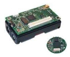
Figure 2.2: Mica motes: Mica2 (left) and Mica2Dot (right)
