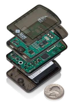
Figure 2.1: A Sun SPOT sensor node and its components
