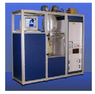
Figure 2.14: Image of a CVD-reactor as used at diamond-materials [17].
