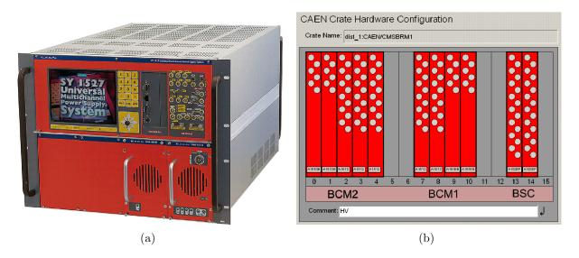
Figure 4.15: CAEN Power Supply System SY1527. a) Crate including controller, connection interfaces and monitor [86]. b) Module layout for BRM systems.
