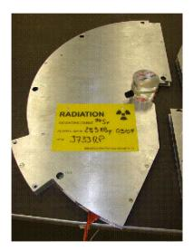
Figure 6.1: Setup used to test all diamond channels of the final system. To generate a signal a  ${}^{90}$ Sr source was put on top of the diamond packages.
