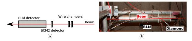
Figure 5.6: SPS beamline setup. a) Schematic, b) photograph (wire chambers are off picture).
