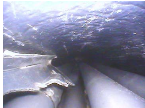
1030 mm, parts of destroyed grid spacer 4
