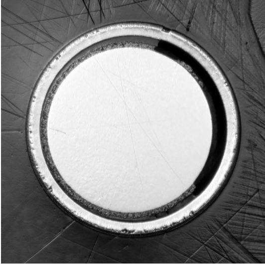
rod 8: Mo coating lost during polishing
