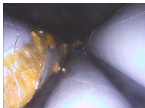
900 mm, traces of Ta_2O_5 (with WO_3 traces) from destroyed TFS 9/13
