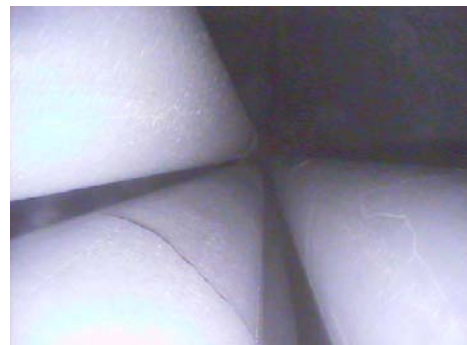
900 mm, circumferential and longitudinal cracks of the fuel rod cladding
