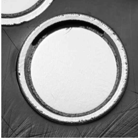
rod 11: Mo coating lost during polishing
