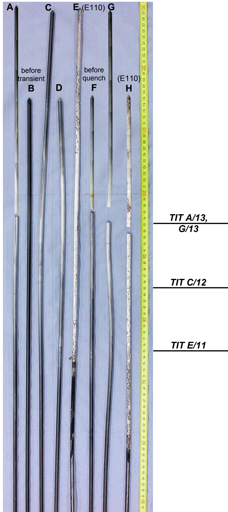
Fig. 35: QUENCH-15; Appearance of withdrawn corner rods B, D, F, H – solid rods; A, C, E, G – tube at lower part (up to TIT position) and solid rod at upper part.
