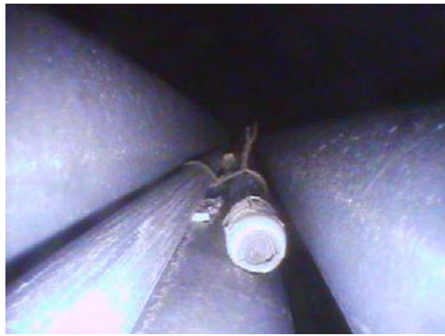
1150 mm, oxidised cap of TFS 9/15
