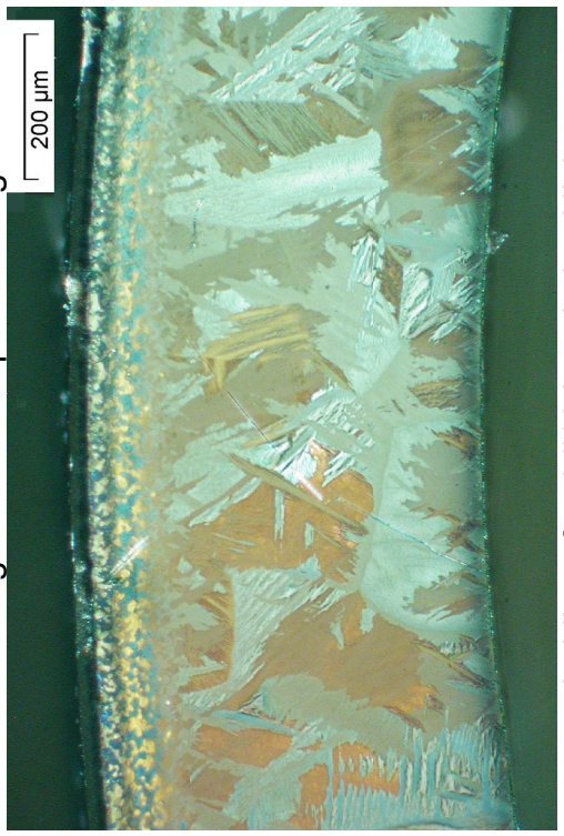
cladding of rod #10 in polarized light
