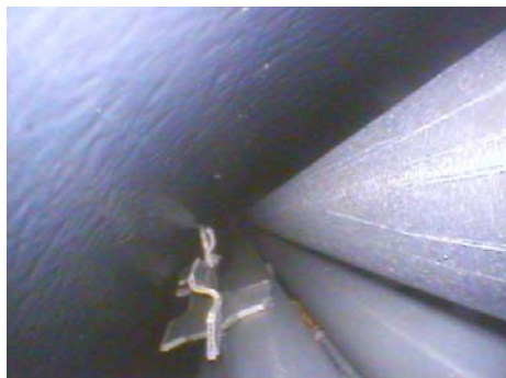
700 mm, relocated part of grid spacer 4
