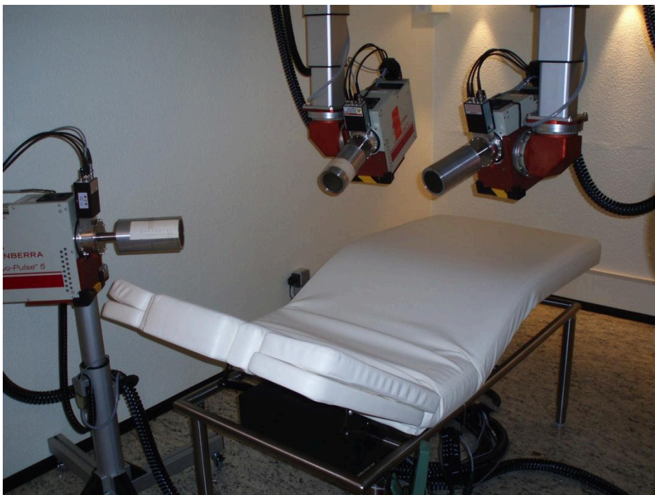
Abb. 4.2: The system (two detectors hanging, one on a cart) ready for a measurement in the whole-body configuration.
