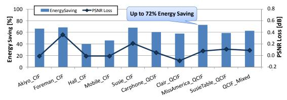
Figure 4.32: Energy and Quality Comparison for the Adaptive Motion Estimator With and Without the enBudget for Various Video Sequences
