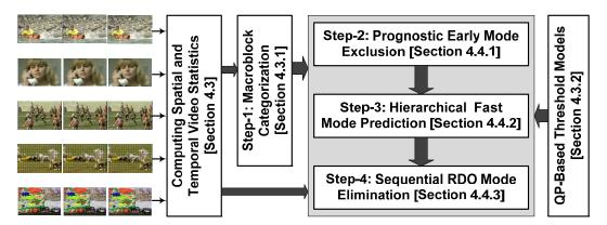
Figure 4.18: Overview of the Adaptive Computational Complexity Reduction Scheme (ACCoReS) showing Different Processing Steps and MB Categorizations
