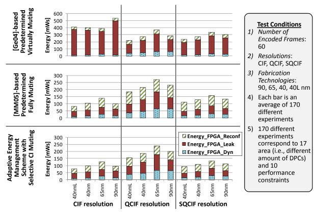
Figure 7.11: Comparing the Energy Breakdown of the Adaptive Energy Management Scheme (with Selective Instruction Set Muting) to [Ge04]-based Pre-VM and [MM05]-based Pre-FM
