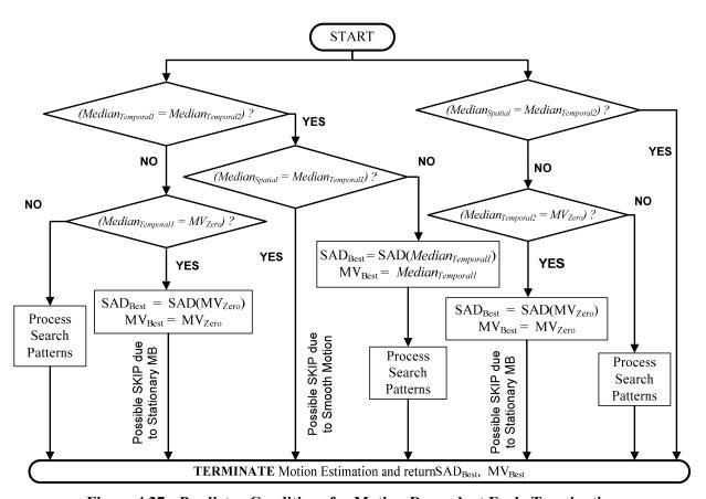
Figure 4.27: Predictor Conditions for Motion-Dependent Early Termination
