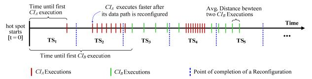
Figure 5.14: Calculating the Weighting Factor for Custom Instructions w.r.t. the Application Context
