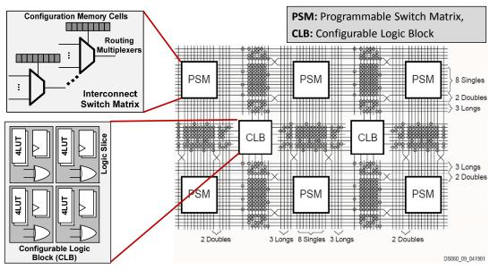
A Typical Composition of a Fine-Grained Reconfigurable Fabric with a 2D-Array of CLBs and PSMs along with the Internal Details of a Spartan-3 Tile [Te06, Xil08a]
