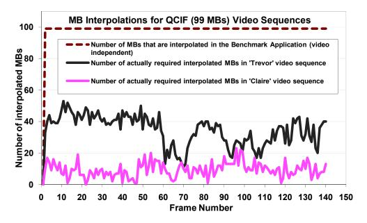
Figure 4.3: Number of Computed vs. Required Interpolated MBs for two Standard Test Sequences for Mobile Devices
