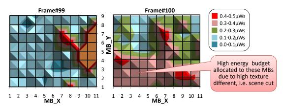
Figure 4.35: Macroblock-Wise Energy Consumption Map of two Exemplary Frames in the SusieTableMix QCIF Sequence for a 90nm Technology
