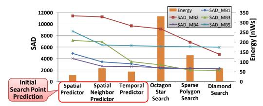
Figure 4.31: SAD vs. Energy Consumption Comparison of different Motion Estimation Stages for Foreman Sequence
