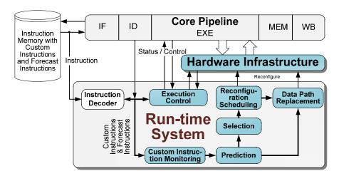
Figure 2.7: Extending a Standard Processor Pipeline towards RISPP and the Overview of the RISPP Run-time System [BSTH07]
