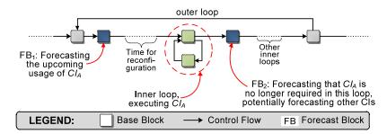
Figure 2.9: Example Control-flow Graph Showing Forecasts and the Corresponding Custom Instruction Executions [Bau09]
