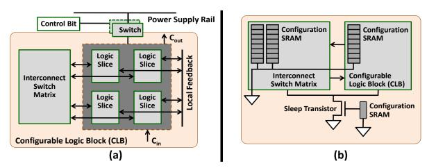
Figure 2.5: State-of-the-Art in Power-Shutdown Infrastructure (a) by [Ge04] (b) by [Te06]
