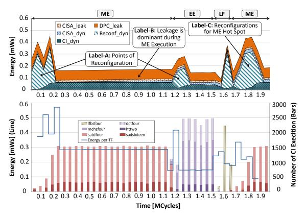
Figure 5.9: CI Execution Results for 30 fps on 65 nm Showing a Detailed Breakdown of Energy Components Highlighting the Contribution of Reconfiguration and Leakage Energy. The Lower Graph Shows the Detailed Execution Pattern of Various CIs Executing in Different Hot Spots of the H.264 Video Encoder Along With Total Energy Consumption
