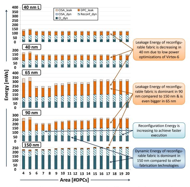
Figure 5.7: Comparison of Energy Components in Different Fabrication Technologies under Various Area Constraints
