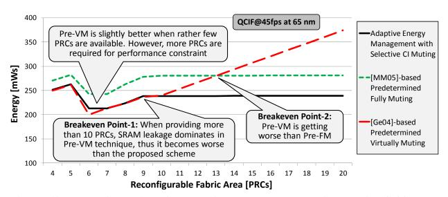
Figure 7.12: Energy Comparison of the Adaptive Energy Management Scheme with [Ge04]-based Pre-VM and [MM05]-based Pre-FM Techniques for Varying Amount of Reconfigurable Fabric
