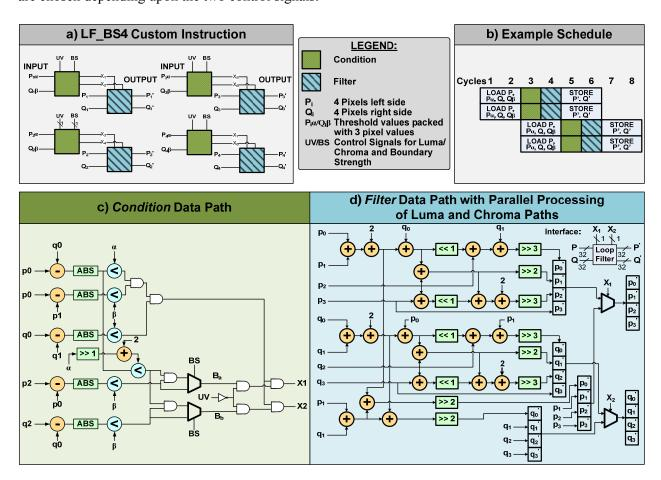
Figure 4.11: Custom Instruction for In-Loop Deblocking Filter with Example Schedule and Constituting Data Paths for Filtering Conditions and Filtering Operation
