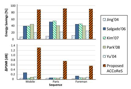
Figure 7.1: Comparing the Energy Savings and Quality Loss of the ACCoReS with Several State-of-the-Art Fast Mode Decision Schemes
