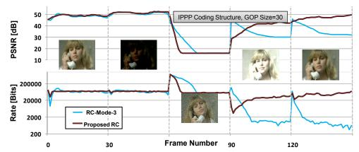
Figure A.9: Frame-wise Comparison of the Multi-Level RC with RC-Mode-0 for Susie Mixed CIF Sequence (Bright, Dark, Noisy) at 2Mbps@30fps
