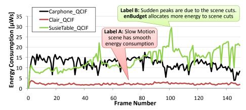
Figure 4.34: Frame-wise Energy Consumption of the Energy-Aware Motion Estimation
