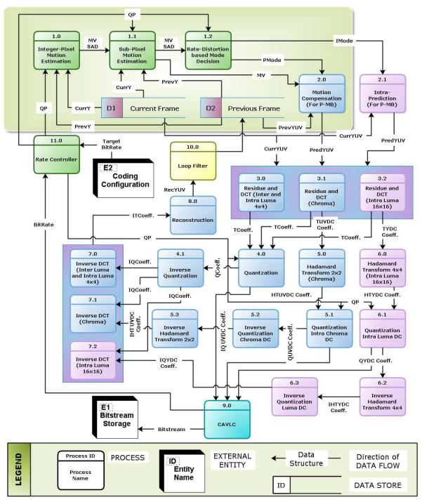
Figure 4.6: Data Flow Diagram of the H.264 Encoder Application Architecture with Reduced Hardware Pressure
