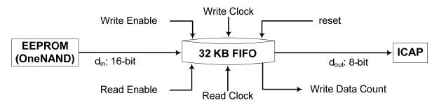
Figure 6.5: Connection of FIFO between EEPROM and ICAP
