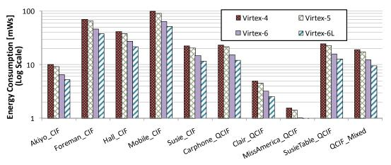
Figure 4.36: Energy Consumption of the Energy-Aware Motion Estimation for Various FPGA Fabrication Technologies for Various Video Sequences
