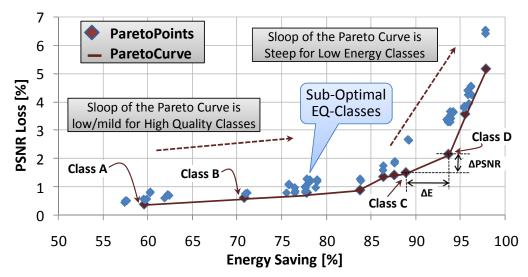
Figure 4.30: Energy-Quality (EQ) Classes: Energy-Quality Design Space Exploration showing various Pareto Points and the Pareto Curve
