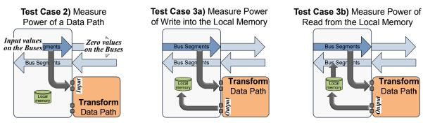
Figure 6.4: Different Test Cases for Measuring the Power of Different Components of a Custom Instruction (CI) Implementation Version
