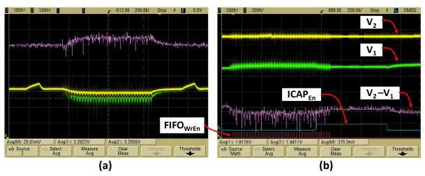
Figure 6.6: (a) EEPROM Voltage Drop while Loading one Data Path Bitstream from EEPROM to FPGA. (b) VCC<sub>INT</sub> Voltage Drop for Transferring one Data Path Bitstream to ICAP and Performing the Corresponding Reconfiguration
