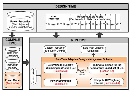
Figure 5.4: Overview of the Proposed Adaptive Low-Power Reconfigurable Processor with Run-Time Adaptive Energy Management along with the Design-, Compile-, and Run-Time Steps
