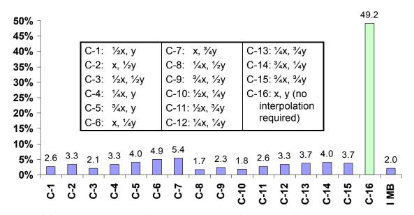
Figure 4.4: Distribution of Different Interpolation Cases in the Carphone Video Sequence
