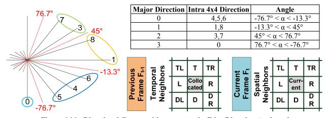
Figure 4.16: Directional Groups with respect to the Edge Direction Angle and Notion of Spatial and Temporal Neighboring Macroblocks
