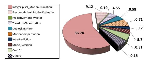
Figure 3.3: Percentage Distribution of Energy Consumption of Different Functional Blocks in the H.264 Video Encoder
