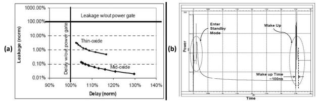
Figure 2.6: (a) Sizing of Thin- & Mid-Oxide Power Gate showing Leakage-Delay Tradeoffs [Te06]; (b) Power Consumption for Activating and Deactivating a single tile [Te06]
