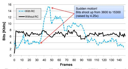
Figure A.1: Comparison of Produced Bits With and Without Rate Control
