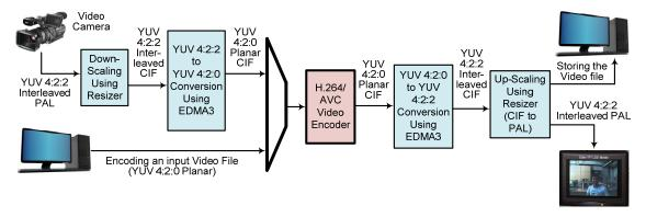
Figure B.5: Flow for porting H.264 Encoder on DM6437 Digital Signal Processor [S.2]
