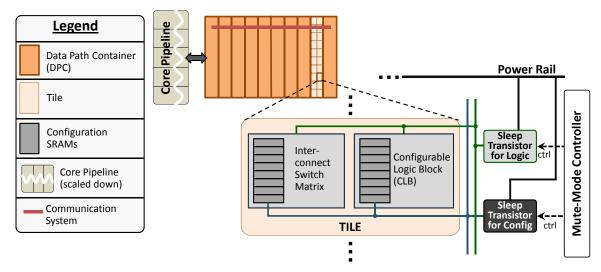
Figure 5.2: Infrastructure Necessary to Exert the Proposed CI Muting Technique
