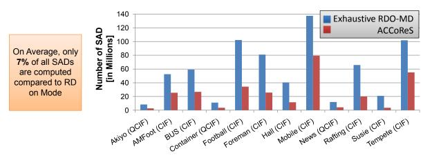
Figure 4.22: Comparison of Total SAD Computations for various video sequences
