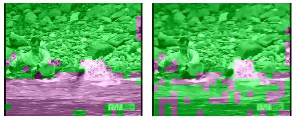
Figure 4.17: Mode Distribution of Frame 4 in Rafting Sequence using the Exhaustive RDO-MD for two different QP values: Left: QP = 16 and Right: QP = 38
