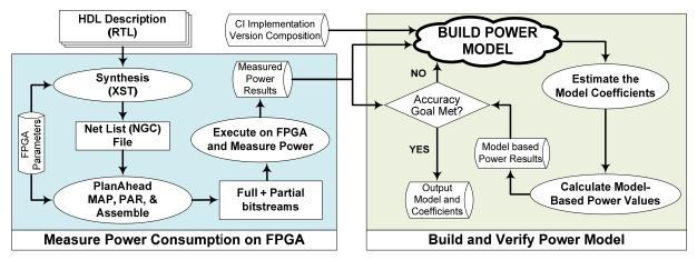
Figure 6.2: Flow for Creating the Measurement-based Power Model
