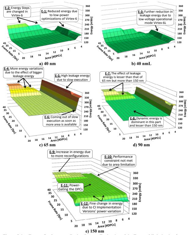
Figure 5.6: Energy-Performance Design Spaces: Evaluation of the Energy Minimization Space Using the Adaptive Energy Management Scheme under Various Area and Performance Constraints for Four Fabrication Technologies for an Encoding of 40 QCIF (176x144) Frames
