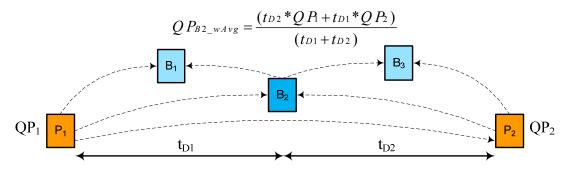
Figure A.4: Temporal Distance based QP Calculation for B Frames/Slices
