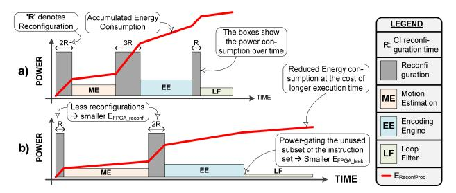
Figure 5.1: Simplified Comparison of Energy Consumption, **Highlighting the Effects of Different Reconfiguration Decisions**
