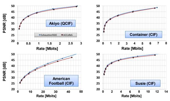
Figure 7.4: Comparing the Rate Distortion Curves for QCIF and CIF Sequences
