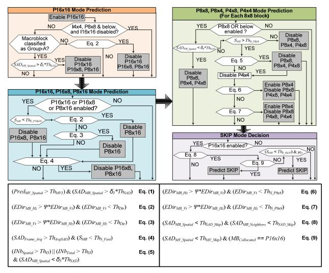
Figure 4.19: Processing Flow of the Hierarchical Fast Mode Prediction
