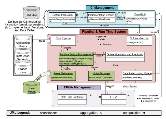
Figure B.2: Reconfigurable Processor Simulator [BSH09a] with the Extensions Implemented in the Scope of this Thesis for Run-Time Adaptive Energy-Management
