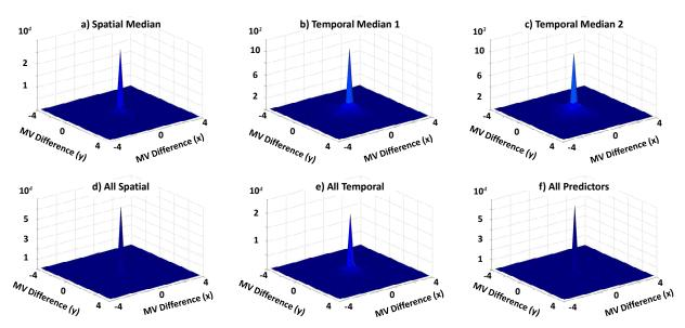
Figure 4.26: Motion Vector Difference Distribution in Foreman Sequence (256 kbps) for Various Predictors Compared to the Optimal Motion Vector (obtained using the Full Search algorithm)
