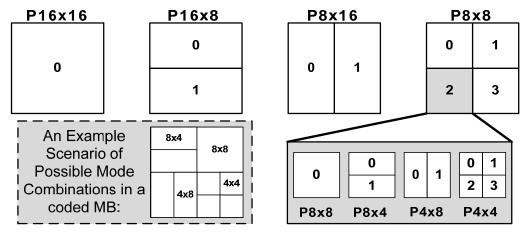
Figure 2.3: Variable Block Sizes for Inter-Predicted MBs (P-MBs) in H.264/AVC
