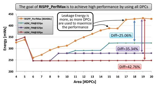
Figure 7.8: Energy Comparison of the AEM FM and RISPP PerfMax schemes for 65 nm
