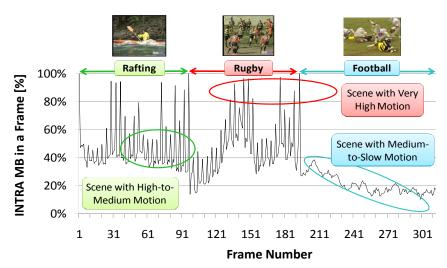
Figure 3.4: Distribution of I-MBs in Slow-to-Very-High Motion Scenes (Test Conditions: Group of Pictures=IPPP..., CAVLC, Quantization Parameter = 28, 30fps)
