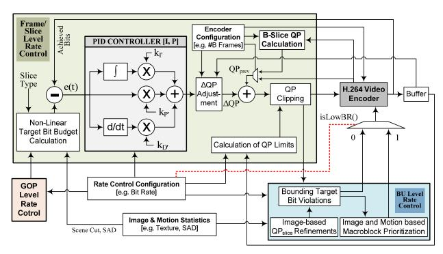
Figure A.2: The Multi-Level Rate Control Scheme covering GOP, Frame/Slice, & BU Levels along with Image and Motion Based Macroblock Prioritization
