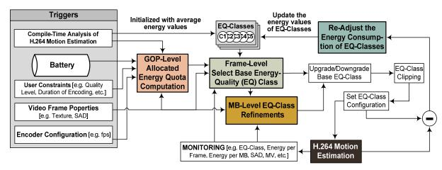
Figure 4.29: Flow of the enBudget Scheme for Energy-Aware Motion Estimation
