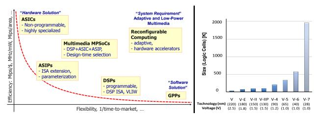
Figure 1.2: (a) Flexibility vs. Efficiency Comparison of Different Architectural Options (inspired from [Hen03]); (b) Evolution Trend of Xilinx Virtex FPGAs [Xil10a]
