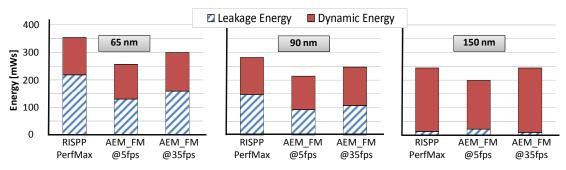
Figure 7.9: Average Energy Comparison of the AEM\_FM and RISPP\_PerfMax for 3 Technologies
