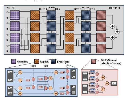
Figure 4.12: Custom Instruction for SATD4x4 showing the Transform and SAV Data Paths
