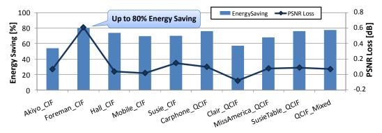
Figure 4.33: Energy and Quality Comparison for the UMHexagonS [CZH02] With and Without the enBudget for Various Video Sequences
