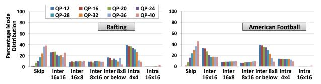
Figure 4.15: Optimal Coding Mode Distribution in Rafting and American Football Sequences at different Quantization Parameter (QP) values
