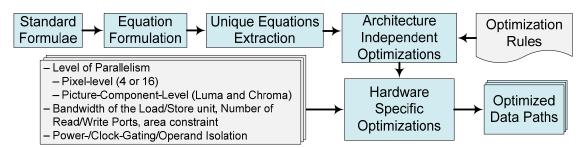
Figure 4.8: Steps to Create Optimized Data Paths from the Standard Formulae
