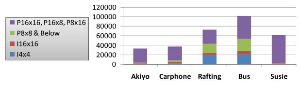
Figure 4.21: Distribution of Mode Processing for QP=28
