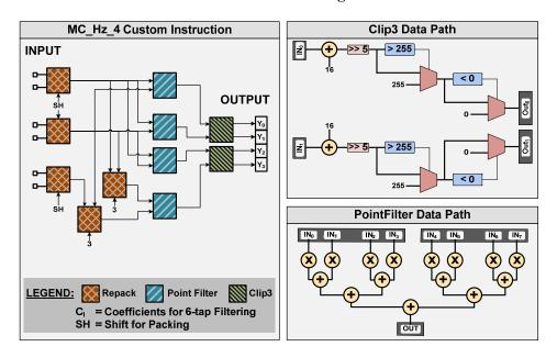
Figure 4.13: Custom Instruction for Motion Compensation showing Different Data Paths
