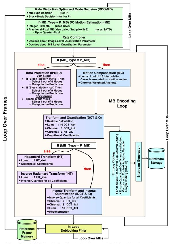
Figure 4.5: H.264 Encoder Application Architecture with Reduced Hardware Pressure
