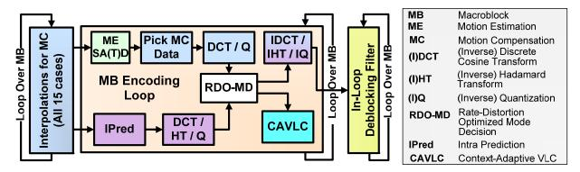
Figure 4.2: Arrangement of Functional Blocks in the H.264 Encoder Benchmark Application
