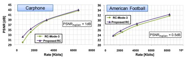
Figure A.6: RD-Curves Comparison of the Proposed Multi-Level RC with RC-Mode-3 for Carphone (QCIF, IPPP) and American Football (SIF, IBBP)
