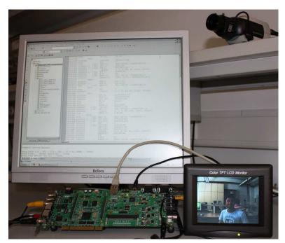
Figure B.4: H.264 Video Encoder Executing on the TI' DM6437 DSP Board [S.2]
