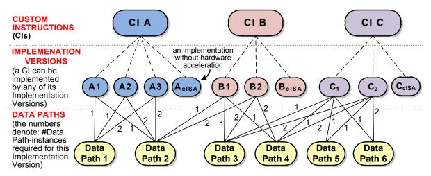
Figure 2.8: Hierarchical Composition of Custom Instructions: Multiple Implementation Versions Exist per Custom Instruction and Demand Data Paths for Realization [BSKH07, BSTH07]
