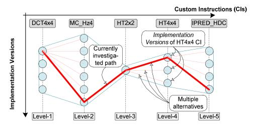
Figure 5.5: Search Space of Five CIs with Their Implementation Versions at the Corresponding Levels and The Path of the Energy-Minimizing Instruction Set
