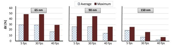
Figure 7.10: Percentage energy saving of Molen [VWG+04] plus AEM\_FM over Molen without AEM\_FM for three technologies
