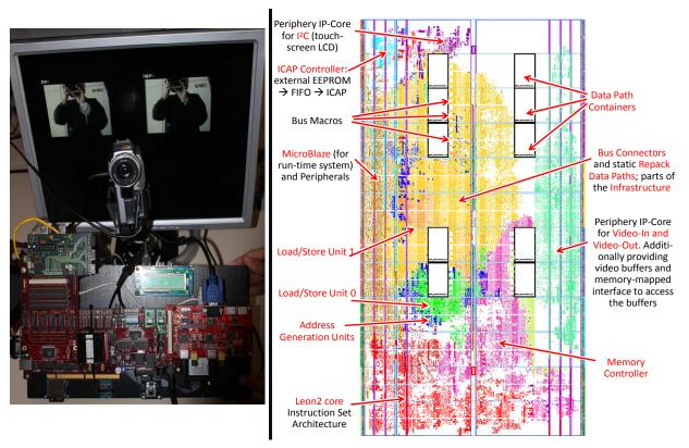
Figure B.3: (A) H.264 Video Encoder Executing on the RISPP Prototype; (B) Floorplan of the RISPP Prototype Implementation on the Xilinx Virtex-4 LX 160 FPGA [Bau09]
