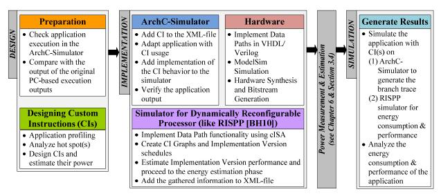
Figure B.1: Simulation Methodology Showing Various Steps of the Simulation Procedure [S.3]
