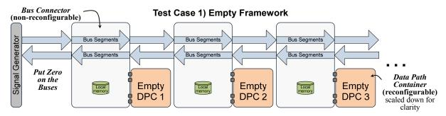
Figure 6.3: Test Case and Setup for Measuring the Power of An Idle (Empty) Framework
