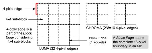
Figure 4.10: 4-Pixel Edges in one Macroblock [ITU05]
