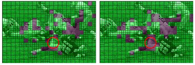
Figure 4.25: MB-level Mode Comparison with the Exhaustive RDO-MD: Frame 17 of American Football. Left: ACCoReS [PSNR=33.28 dB], Right: Exhaustive RDO-MD [PSNR=34.52 dB]
