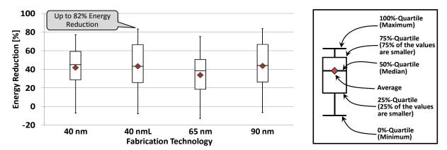
Figure 7.13: Energy Savings of the Adaptive Energy Management Scheme Compared to the [Ge04]-based Pre-VM technique
