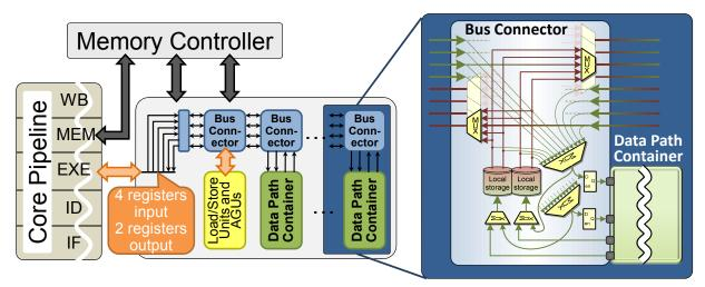
Figure 2.11: Overview of the Hardware Infrastructure for Computation (Data Path Container) and Communication (Bus Connector) showing the Internal Composition of a Bus Connector [Bau09]
