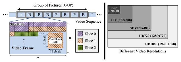
Figure 2.1: An Overview of the Digital Video Structure (showing Group of Pictures, Frame, Slice, MB) and Different Video Resolutions
