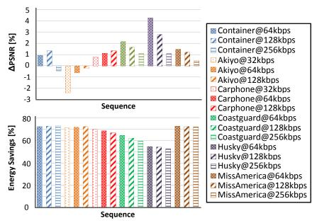
Figure 7.3: Energy Savings and Quality Loss of the ACCoReS compared to the Exhaustive RDO-MD for QCIF Resolution Video Sequences
