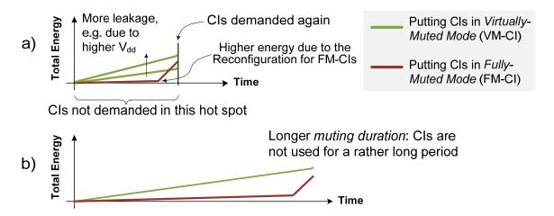
Figure 5.10: Comparing the Energy Requirements of Virtually- & Fully-Muted CIs for 2 Scenarios
