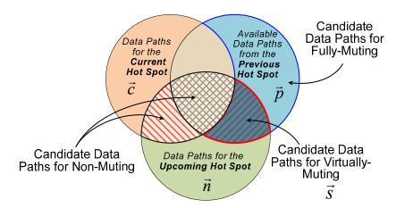
Figure 5.13: Venn Diagram Showing the Data Path Requirements of **Previous, Current, Upcoming Hot Spots**
