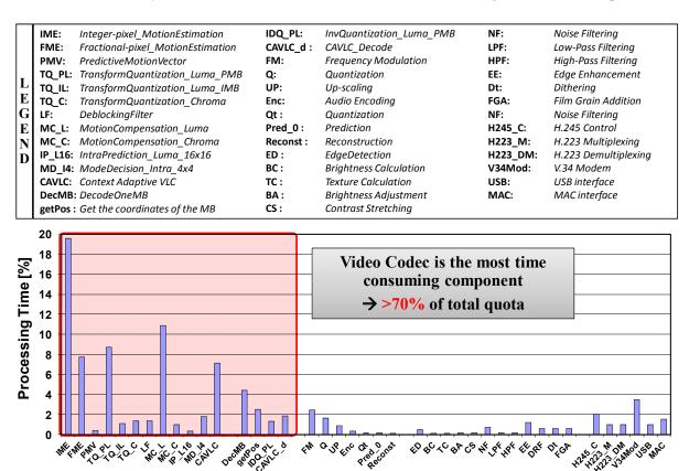
Figure 3.2: Processing Time Distribution of Different Functional Blocks in the H.324 Video Conferencing Application
