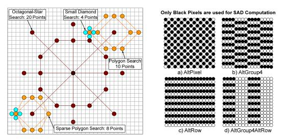
Figure 4.28: Four Search Patterns used in the Adaptive Motion Estimator and the Pixel-Decimation Patterns for SAD Computation
