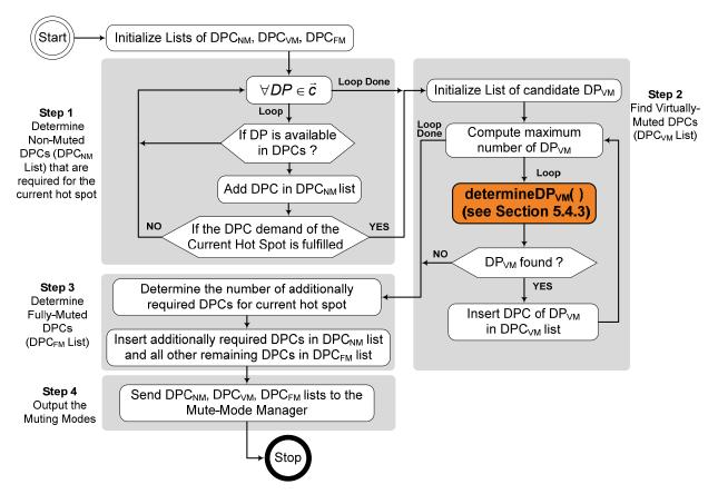
Figure 5.12: Flow for Selecting a Muting Mode for the Custom Instruction (CI) Set
