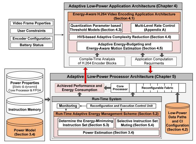
Figure 3.5: Overview of the Adaptive Low-Power Application and Processor Architectures
