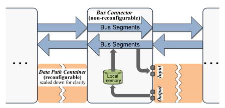
Figure 3.7: Power-Relevant Components of the Computation- and Communication Infrastructure to Execute CI Implementation Versions [BSH08a]
