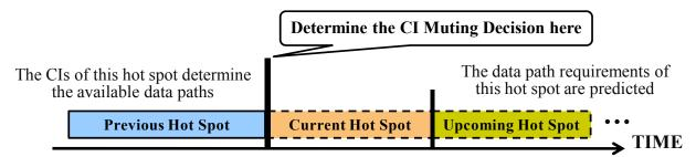
Figure 5.11: Time-line showing the execution sequence of hot spots and the situation for a CI Muting decision
