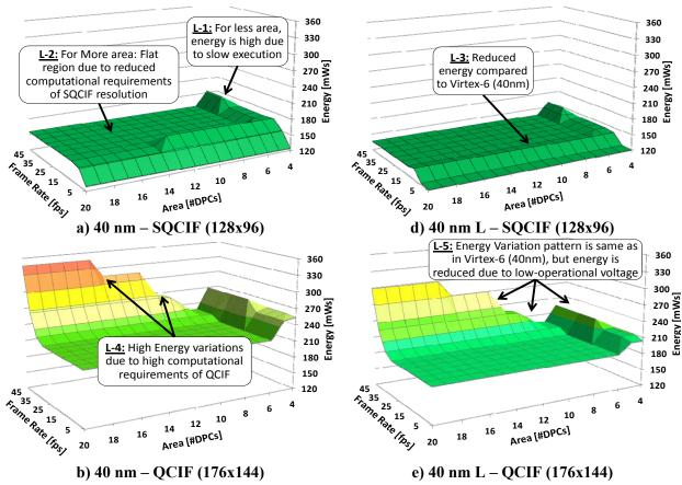
Figure 5.8: Comparing Energy-Performance Design Spaces for Different Video Resolutions when using the Energy Management Scheme under Various Area and Performance Constraints for an Encoding of 60 Video Frames
