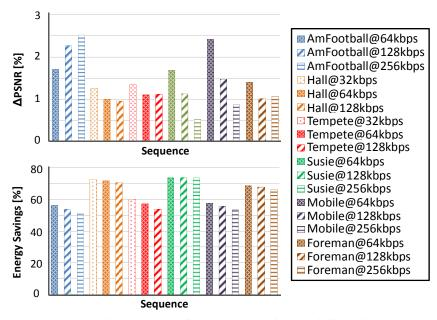
Figure 7.2: Energy Savings and Quality Loss of the ACCoReS compared to the Exhaustive RDO-MD for CIF Resolution Video Sequences
