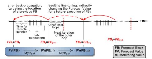
Figure 2.10: Execution Sequence of Forecast and Custom Instructions with the Resulting Error Back Propagation and Fine-tuning [Bau09]
