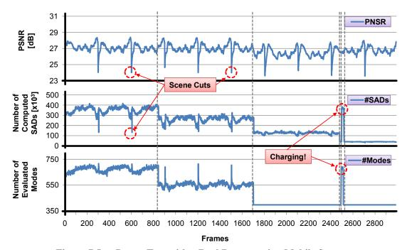
Figure 7.5: Power Test with a Real Battery using Mobile Sequence
