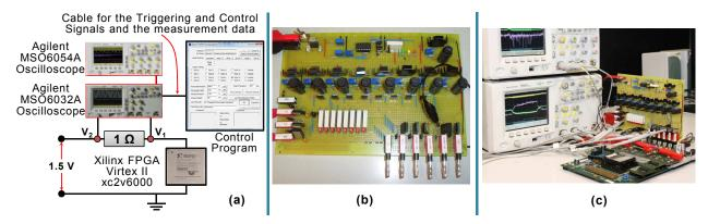
Figure 6.1: a) Measurement setup, b) the in-house Developed Power Supply board
