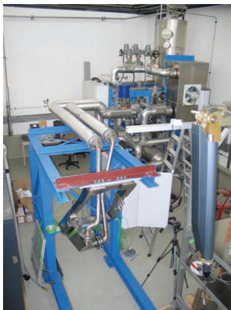
LHT test facility with BSM corner prototype mock-up
