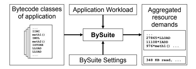
Figure 4.1.: High-level overview of Resource Demand Quantification in BYCOUNTER
