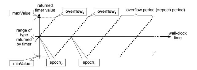
Figure 3.11.: Overflow of range-limited values
