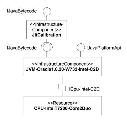
Figure 6.6.: Initial Modelling of the Calibration Factor as a Separate Infrastructure Component
