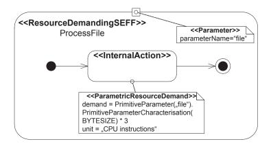
Figure 6.1.: PCM RDSEFF with one internal action
