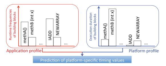
Figure 1.4.: Overview of the cross-platform performance prediction approach of this thesis
