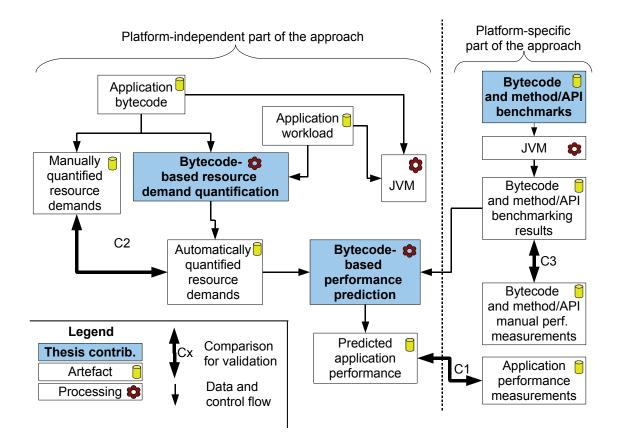
Figure 7.1.: Validation of Bytecode-based Performance Prediction (Overview)
