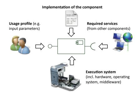
Figure 1.1.: Performance of software components: influencing factors
