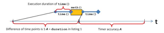
Figure 3.5.: Accuracy is larger than timer method execution duration, measured duration too large
