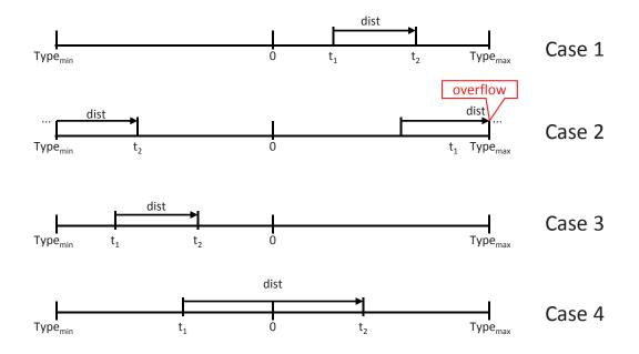
Figure 3.12.: The impact of numeric ranges on measuring time intervals between  $t_1$  and  $t_2$
