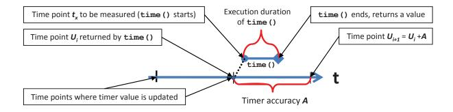
Figure 3.3.: Effects of timer accuracy on measurements (Legend:  $t_x$ : actual time to be measured;  $U_i$ : counter updates; A: timer method accuracy)
