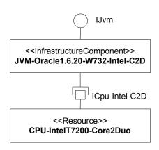
Figure 6.5.: Specialising CPU Resource Interfaces to Model Platform-Dependent JVM Benchmarking Results (the squared interface is a resource interfaces)
