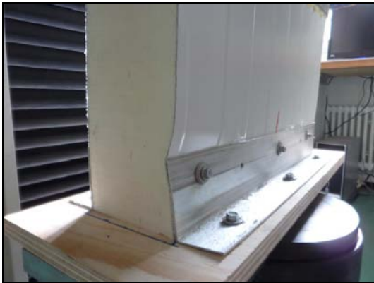
failure at the lower end
