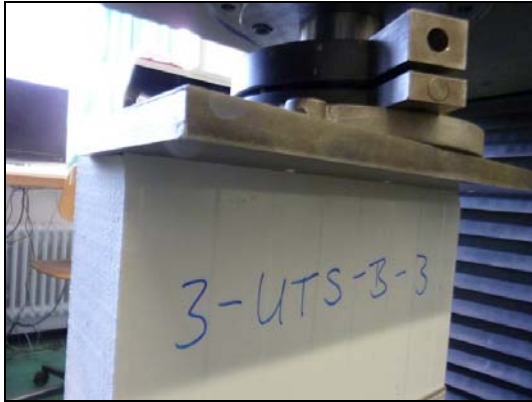
Failure of the stressed face
