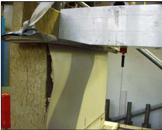
Failure of the stressed face
