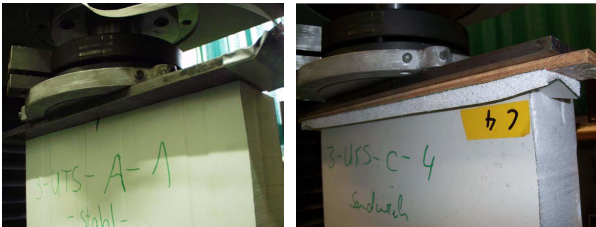
Fig. 9: Introduction of load by plate of steel and by sandwich panel
