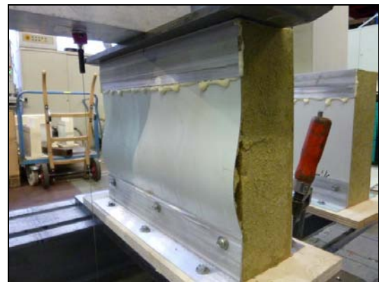
buckling of the compressed face
