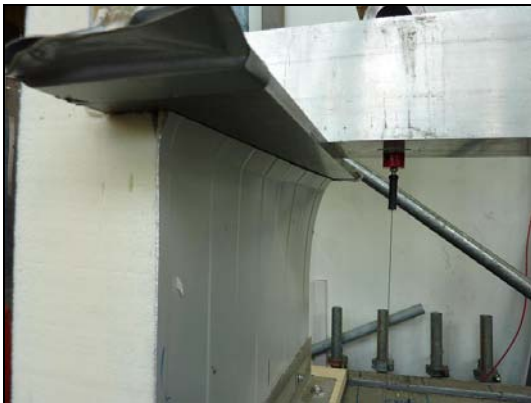
Failure of the stressed face
