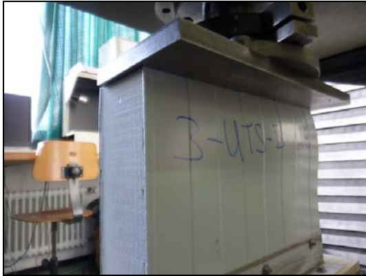
Failure of the stressed face
