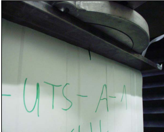
Crippling of the stressed face
