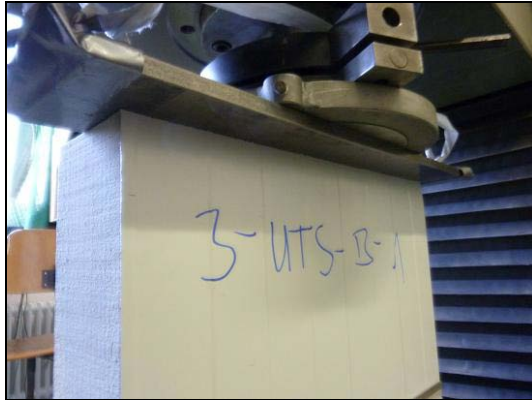
Failure of the stressed face
