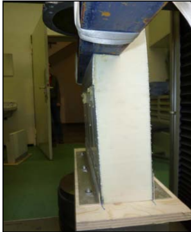
deformation prior to failure
