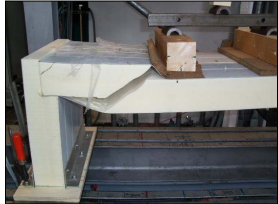
shear failure of the ceiling panel
