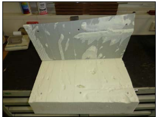
bond between face and core
