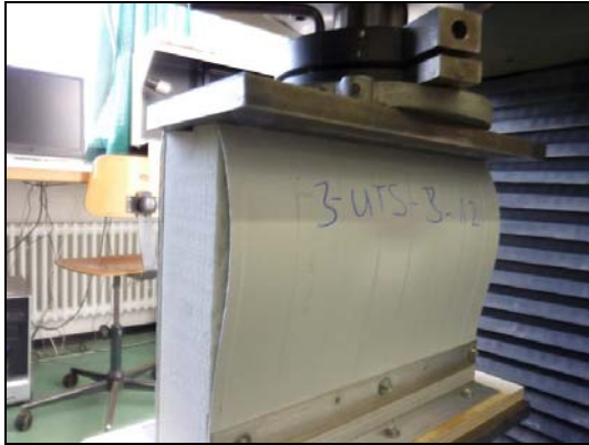
Failure of the stressed face
