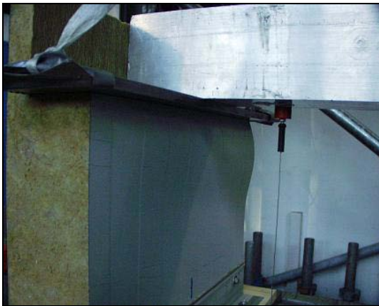
Failure of the stressed face
