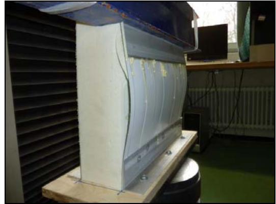
failure of the compressed face
