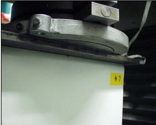
Failure of the stressed face
