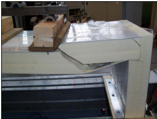
shear failure of the ceiling panel
