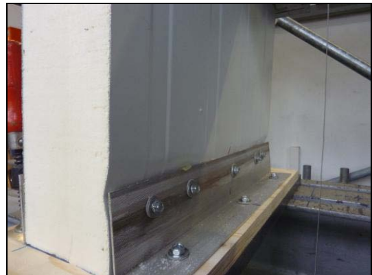
failure of the lower end
