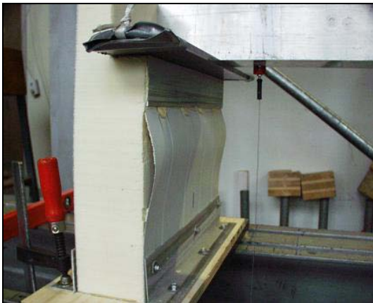
failure of the compressed face
