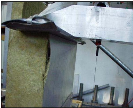
Failure of the stressed face
