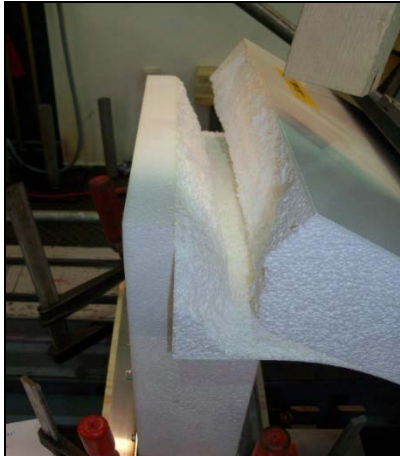
failure of core material
