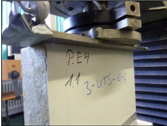
Failure of the stressed face
