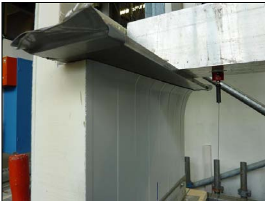
Failure of the stressed face
