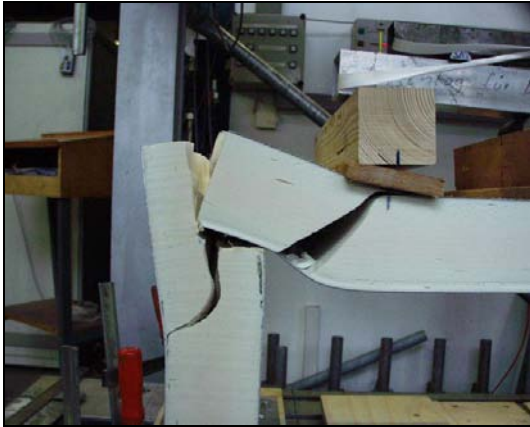
shear failure of the ceiling panel
