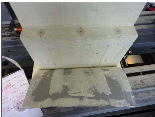
bond between face and core
