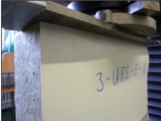
Failure of the stressed face
