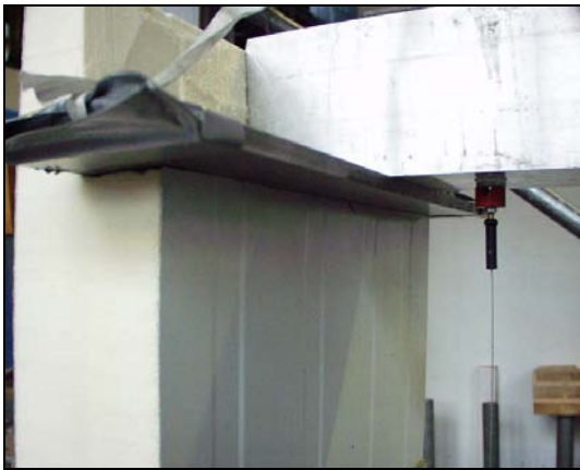
Failure of the stressed face
