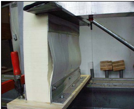
failure of the compressed face
