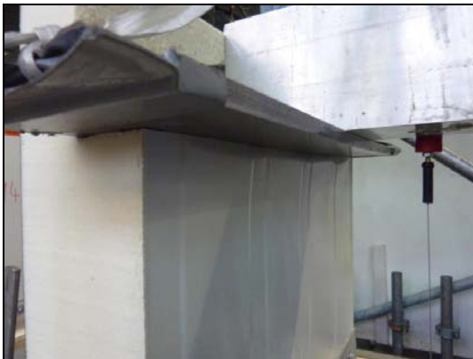
Failure of the stressed face
