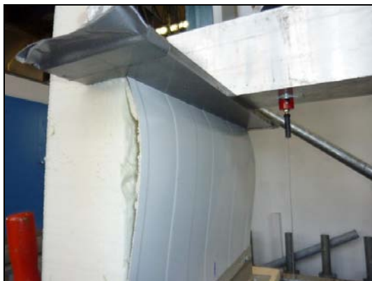
Failure of the stressed face
