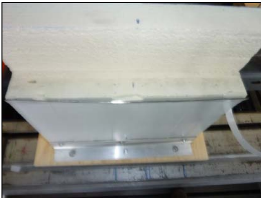
Failure of the stressed face
