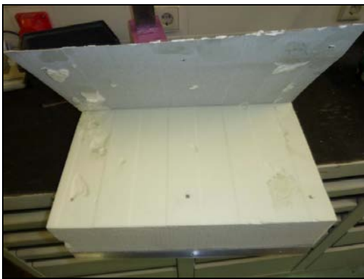
bond between face and core
