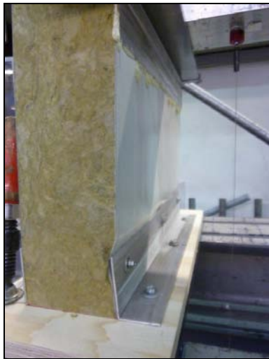
failure of the lower end
