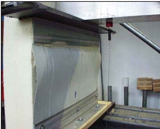
failure of the compressed face
