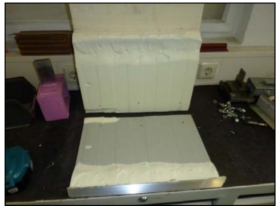
bond between face and core
