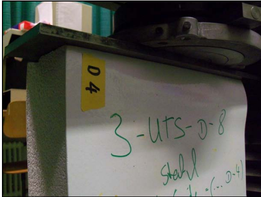
Failure of the stressed face
