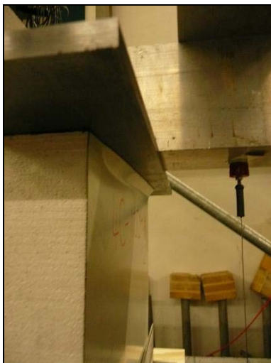
Failure of the stressed face
