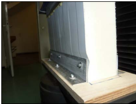
failure at the lower end
