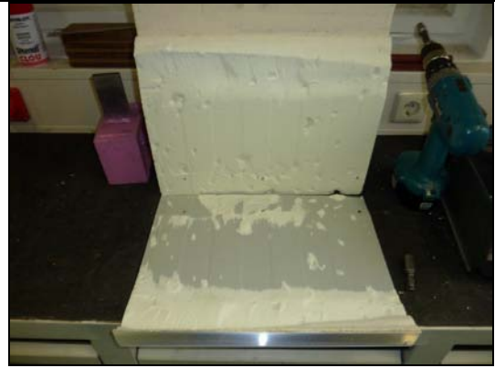
failure of the compressed face
