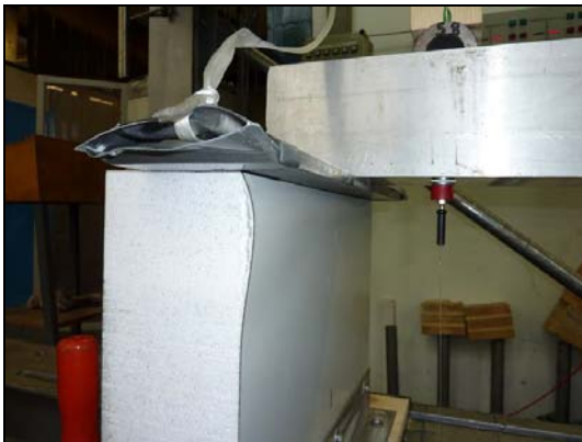
Failure of the stressed face
