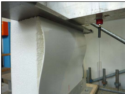
failure of the compressed face
