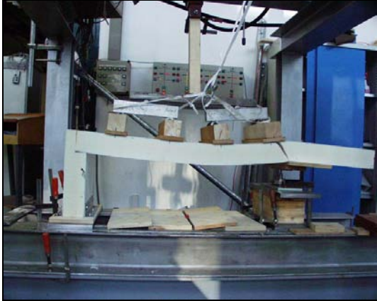
shear failure of the ceiling panel
