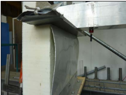
Failure of the stressed face
