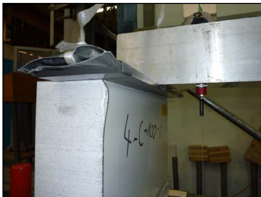
Failure of the stressed face
