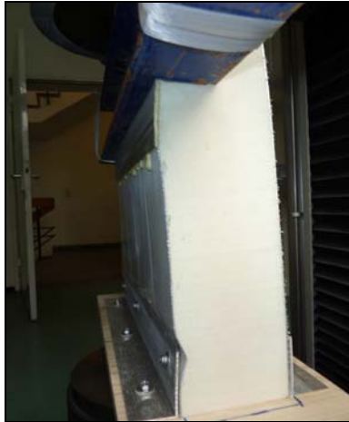
failure at the lower end
