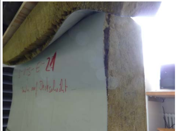
Failure of the stressed face
