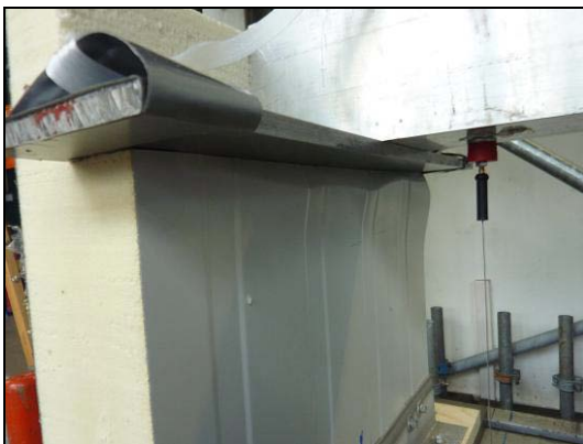
failure of the compressed face
