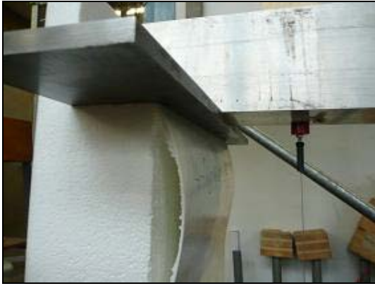
Failure of the stressed face
