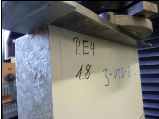
Failure of the stressed face
