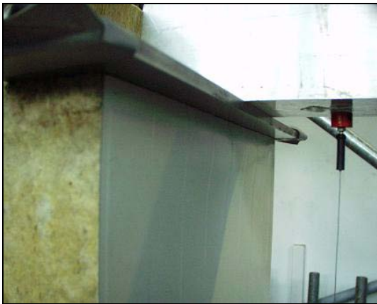
Failure of the stressed face
