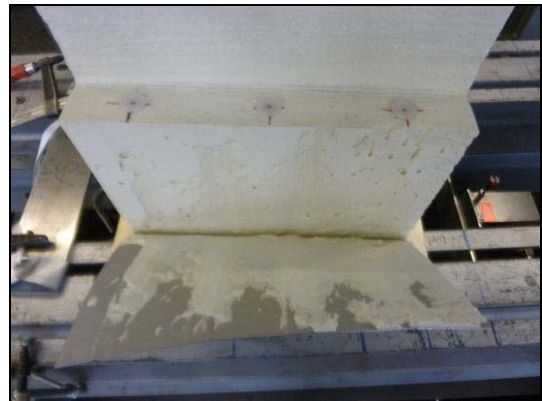
bond between face and core
