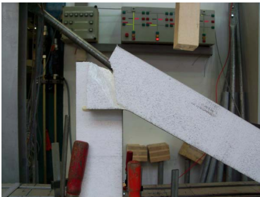
failure of core material
