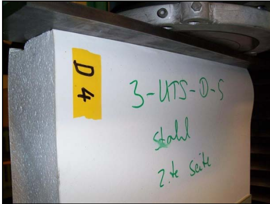
Failure of the stressed face
