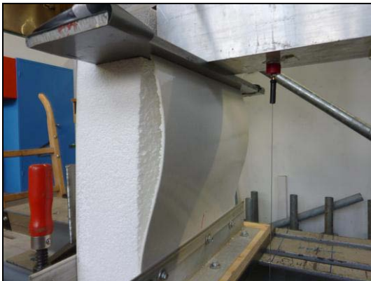
failure of the compressed face
