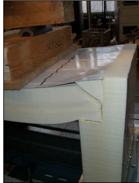
failure of glued corner detail
