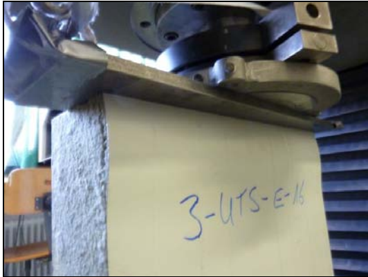
Failure of the stressed face
