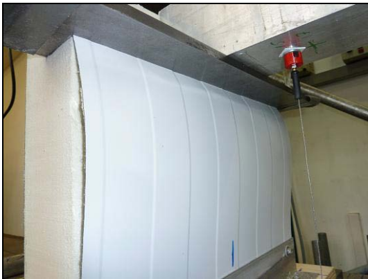
Failure of the stressed face
