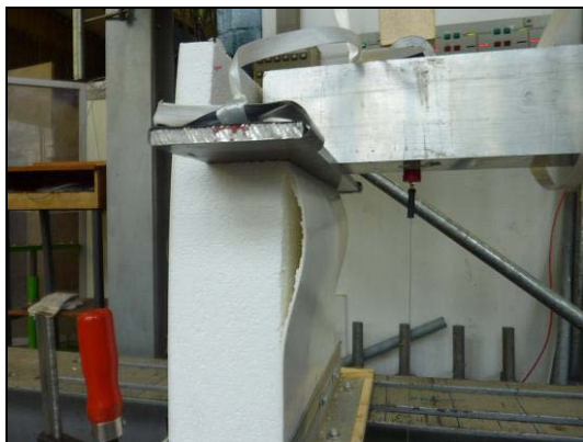
failure of the compressed face
