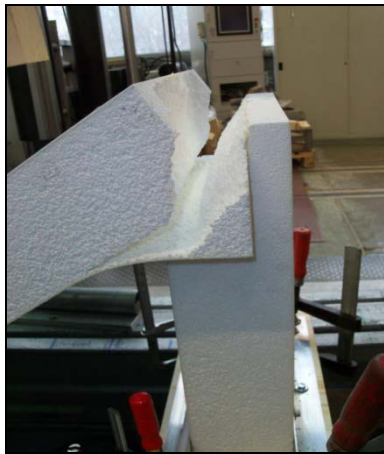
failure of core material
