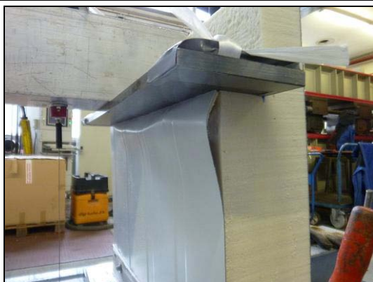
failuer of the compressed face
