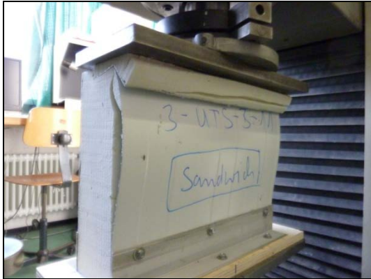
Failure of the stressed face
