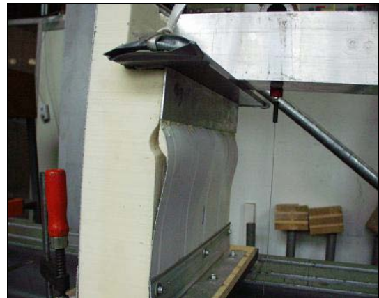
buckling of the compressed face
