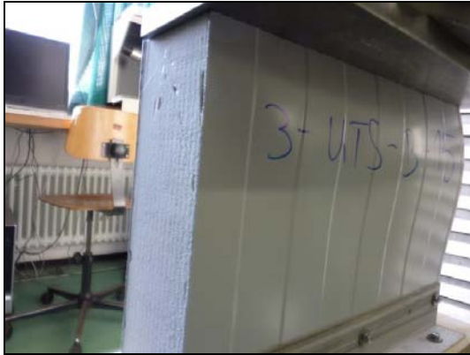
Failure of the stressed face
