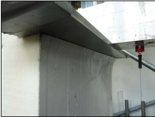
Failure of the stressed face
