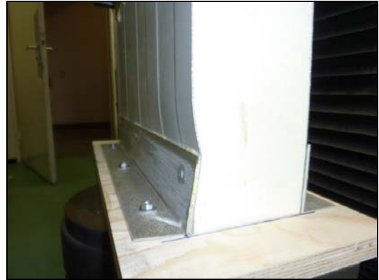
failure at the lower end
