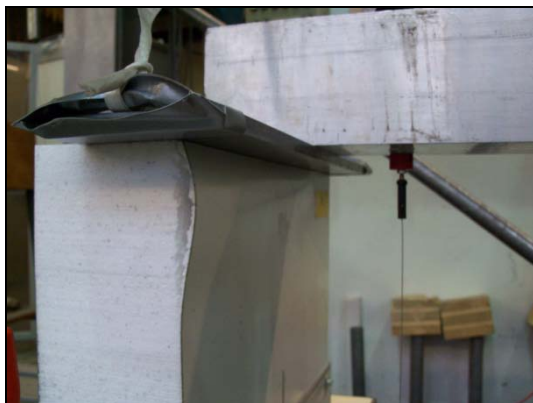
Failure of the stressed face
