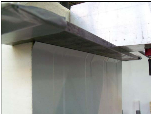
Failure of the stressed face
