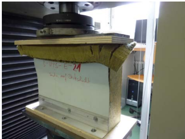
Failure of the stressed face
