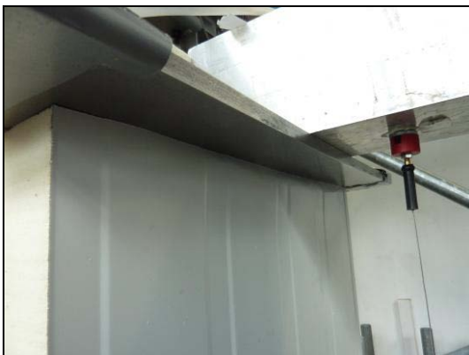
failure of the compressed face
