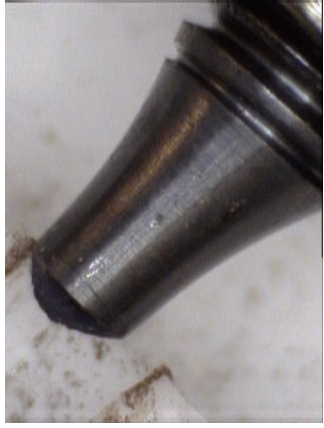
Fig. 10-17 Photographs (macro) of the tensile tested EUROFER 97 specimens: E1 09 ( T_{\text{test}}=350\text{ }^{\circ}\text{C} after annealing at 550\text{ }^{\circ}\text{C}/1\text{ h} ), E1 34 ( T_{\text{test}}=20\text{ }^{\circ}\text{C} ), E1 35 ( T_{\text{test}}=350\text{ }^{\circ}\text{C} ).
