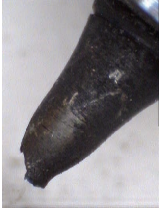
Fig. 10-25 Photographs (macro) of the tensile tested OPTIFER XII specimens: 12 01 ( T_{\text{test}}=20\text{ }^{\circ}\text{C} ), 12 02 ( T_{\text{test}}=350\text{ }^{\circ}\text{C} ), 12 03 ( T_{\text{test}}=350\text{ }^{\circ}\text{C} after annealing at 550\text{ }^{\circ}\text{C}/3\text{ h} ).
