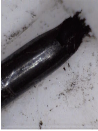
Fig. 10-28 Photographs (macro) of the tensile tested EURODSHIP (EUROFER ODS with 0.5 wt.% Y_2O_3 ) specimens: EO 29 ( T_{test}=20\text{ }^\circ\text{C} ), EO 30 ( T_{test}=350\text{ }^\circ\text{C} ).
