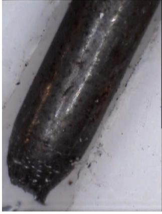
Fig. 10-20 Photographs (macro) of the tensile tested F82H-mod. specimens: F 06 ( T_{\text{test}}=350\text{ }^{\circ}\text{C} ), F 07 ( T_{\text{test}}=350\text{ }^{\circ}\text{C} ), F 08 ( T_{\text{test}}=20\text{ }^{\circ}\text{C} ).
