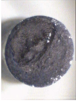
Fig. 10-17 Photographs (macro) of the tensile tested EUROFER 97 specimens: E1 09 ( T_{\text{test}}=350\text{ }^{\circ}\text{C} after annealing at 550\text{ }^{\circ}\text{C}/1\text{ h} ), E1 34 ( T_{\text{test}}=20\text{ }^{\circ}\text{C} ), E1 35 ( T_{\text{test}}=350\text{ }^{\circ}\text{C} ).
