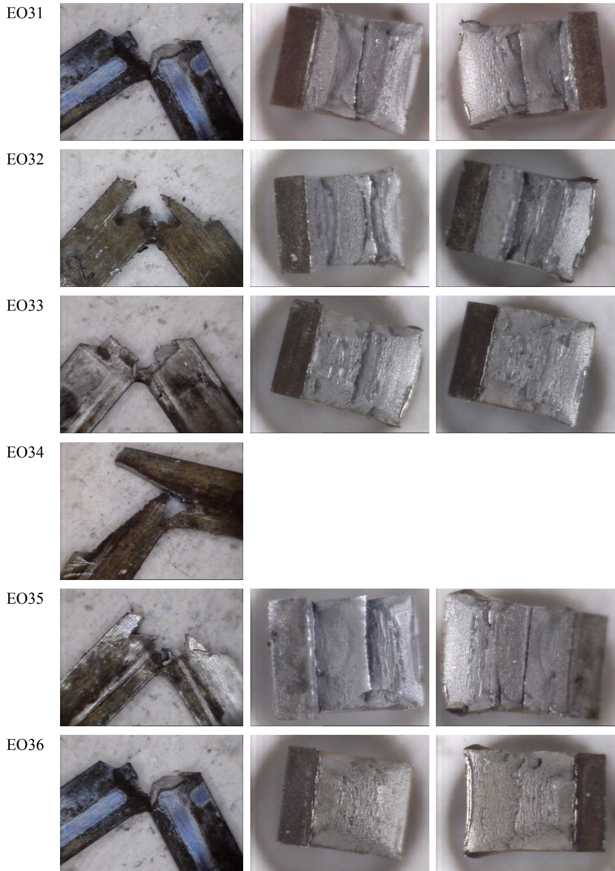
Fig. 9-25 Charpy specimens EO 31, EO 32, EO 33, EO 34, EO 34, EO 36 after impact testing and after complete separation.
