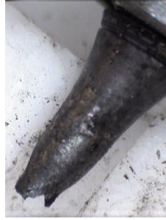
Fig. 10-22 Photographs (macro) of the tensile tested ADS 3 specimens: A3 01 ( T_{\text{test}}=20\text{ }^{\circ}\text{C} ), A3 02 ( T_{\text{test}}=350\text{ }^{\circ}\text{C} ), A3 03 ( T_{\text{test}}=350\text{ }^{\circ}\text{C} after annealing at 550\text{ }^{\circ}\text{C}/3\text{ h} ).
