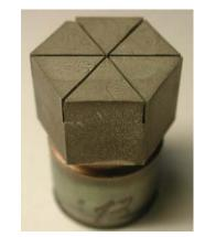
Figure 3.9-15: Second HHF test series, mock-up #13 (HEMJ, castellated).
