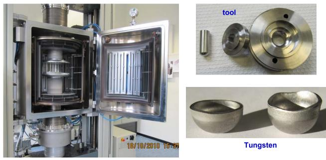
**Figure 4.3-3:** Successful deep-drawing tests with 1 mm W-sheet. Left: Vacuum furnace (courtesey V. Toth/KIT); Top right: newly developed tool made of tool steel; Bottom right: two deep-drawn W thimble-like caps (Ø15 x 1) of about 8 and 11 mm height, respectively.
