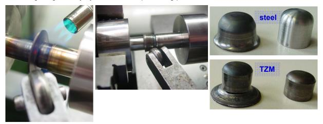
**Figure 4.3-2:** Roll pressing attempt using butane gas heating (left), thimble cap from 1 mm sheet of steel and TZM (right) [4.1-2]. Image courtesy of J. Reiser.
