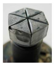
Figure 3.9-29: Third HHF test series, mock-up #32. Image after tests (10 cycles at q=10  $\rm MW/m^2).$
