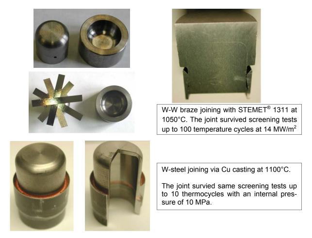
**Figure 3.9-5:** First successful attempts in joining of W parts with curvature (top) using a Nibased filler metal STEMET<sup>®</sup> 1311 and W-steel parts with copper filler (bottom). Courtesy of Efremov.
