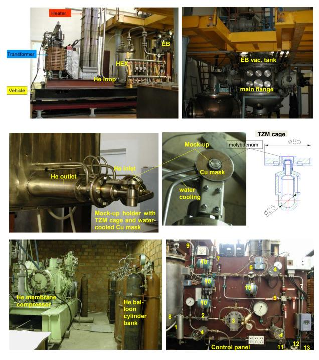
**Figure 3.9-2:** Built-in components of the helium loop and the TSEFEY vacuum tank. Control panel: 1 – filter, 2 – throttling orifice for gas flow measuring, 3 – gas pressure regulator (output pressure 10 MPa), 4 – motorized valve, 5 – manual valve, 6 –gas flow regulator, 7 – safety valve, 8 – heater line, 9 – cooler line, 10 – measuring differential pressure, 11 – to feeding balloon cylinder bank, 12 – to vacuum line, 13 – to receiving balloon cylinder bank.
