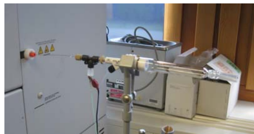
Fig. 2: Set-up of capillary, nebulizer, and spray chamber (Mira Mist CE system) used for the CE-SF-ICP-MS measurements.
