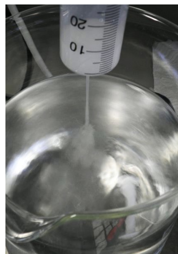
(c) Diluting sampled mother solution; Pivoting of the syringe prevented clogging in case of strong crystallization in syringe. Also, dipping the syringe tip in the water enhanced evacuation.
