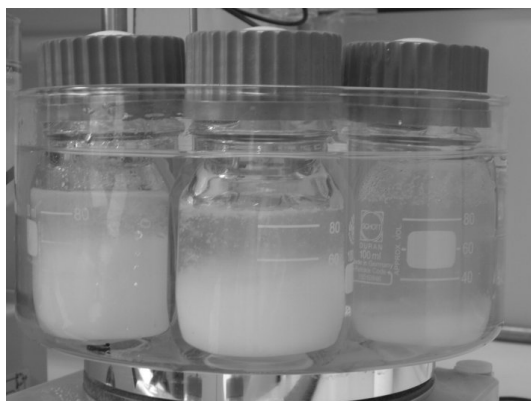
(a) Equilibration vessels with different salt concentrations in oil bath; here: 75, 85 and 90% at 80^\circ\text{C} (from left to right); The indicated concentrations refer to % \text{H}_2\text{O} evaporated with respect to the initially simulated concentration.
