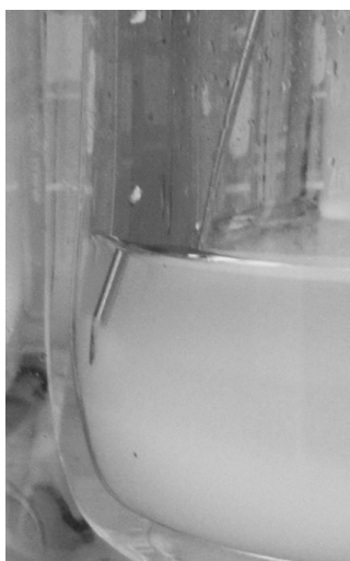
(a) Needle in equilibration vessel; If crystals are big (e.g. in case of crystallization, i.e. coming from above, or long equilibration time), a crystal cloud forms around the syringe tip, which decreases the amount of crystals sucked in.
