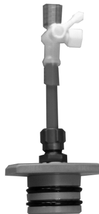
(b) Vacuum adapter with valve manufactured by Eawag workshop
