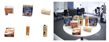
Fig. 5.3. Object candidate detection in the peripheral cameras. Left: Views of the target objects are trained and matched with the scene. Right: Typical scene for detection queries.
