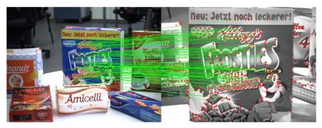
Fig. 5.15. Purged correspondences after applying the Hough transform to the matches. The illustrated matches correspond to the bin in Hough space with maximum vote.
