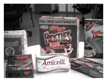
Fig. 5.12. Harris corner points extracted in the foveal camera image with a minimum cornerness of  $C_{min} = 0.001$ .
