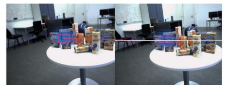
Fig. 5.10. Calculation of stereo correspondences for object candidates. In each image of the stereo camera pair candidate regions are extracted using the CCH descriptor. Using the center of regions in the left image, the epipolar line in the right image is calculated (white). For regions in the right image that intersect the epipolar line, correspondences are calculated using correlation techniques (red).
