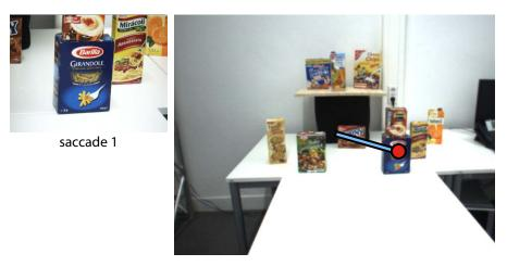
Fig. 9.4. Scan pattern in the pasta box search task. The pasta box (object 6) could be brought to the foveal cameras with a single saccade in all test cases.
