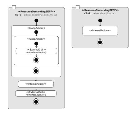
Figure 5.13.: RDSEFFs for the coarse-grained components C2-1 and C2-2
