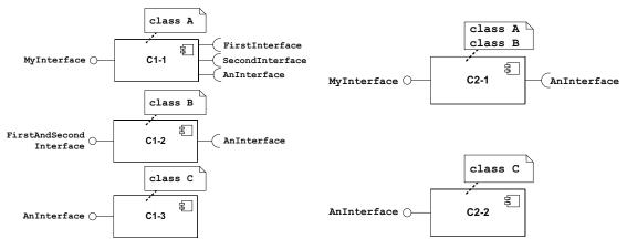
(a) Classes A, B, and C as separate components (b) Classes A and B merged into a single component
