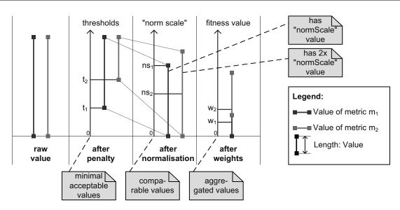
Figure 5.23.: Thresholds reflect lower boundaries; normalisation reflects typical upper values; the fitness value aggregates multiple metrics after weighting them
