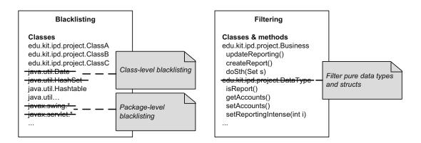
Figure 4.7.: Blacklisting and filtering
