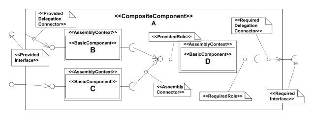
Figure 2.4.: Example: PCM composite component (from [Koz08b])
