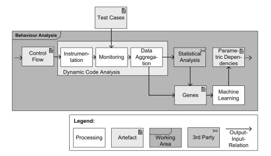
Figure 5.14.: Dynamic analysis: Excerpt of behaviour analysis
