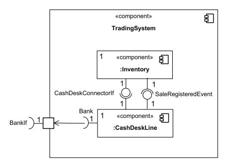
Figure A.1.: CoCoME System Level Architecture, source [HKW<sup>+</sup>08]
