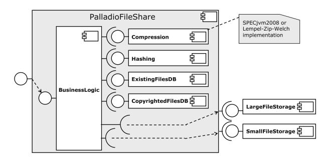
Figure A.6.: Palladio FileShare Static Architecture, source [KKR08a]
