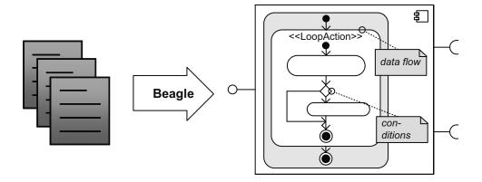
Figure 5.1.: The *Beagle* approach reverse engineers behavioural models of component services
