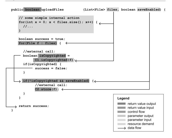
Figure 2.6.: Parametric dependencies in code at a component abstraction level
