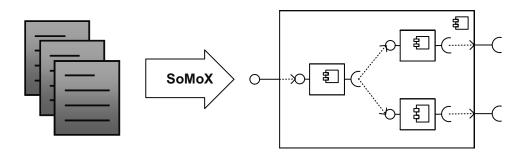
Figure 4.1.: The *SoMoX* approach reverse engineers a static component-based architecture from source code.
