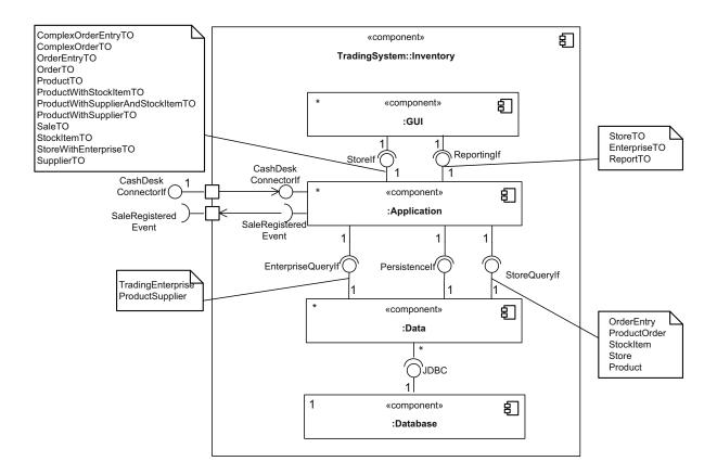
Figure A.2.: CoCoME Inventory: Subsystem Level Architecture, source [HKW<sup>+</sup>08]
