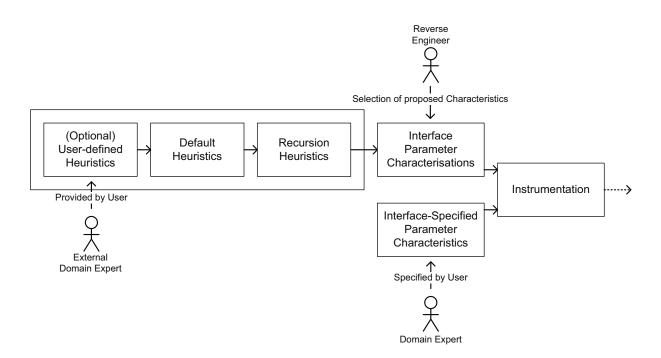
Figure 5.16.: Heuristics for selection of parameter characterisations
