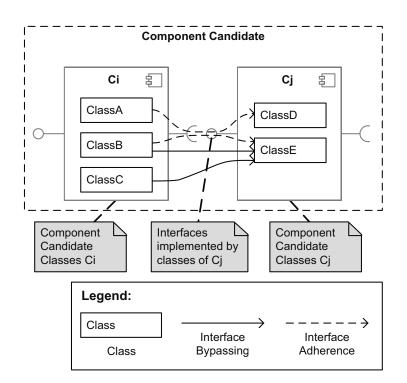
Figure 4.9.: Example: Interface adherence and bypassing
