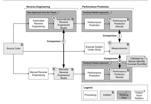
Figure 7.1.: Overview on the validation purposes in the Palladio context: Reverse engineering (left), performance prediction (right)
