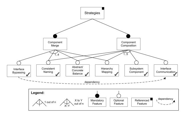
Figure 4.4.: Feature diagram of strategies for merging and composing Components
