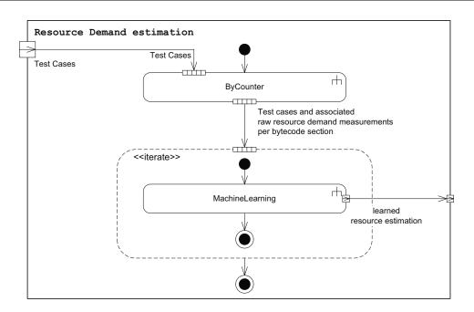
Figure 5.32.: UML activity diagramm: Integration of resource demand counting ("ByCounter") in the reverse engineering process of behavioural models
