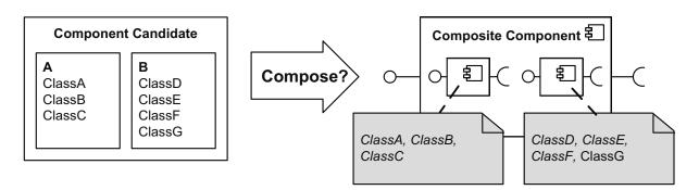
Figure 4.12.: The component composition strategy indicates when to create a new composite component from a component candidate
