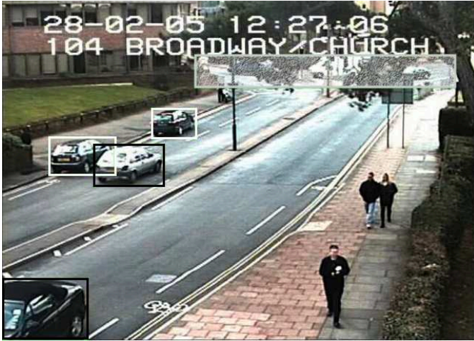
Fig. 3. Sample annotation for vehicle. MOBILE objects are marked by black boxes. STATIONARY objects are marked by white boxes. The shaded region indicates where mobile vs. stationary is ambiguous.
