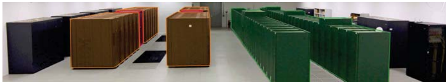
Figure 32: The high-performance supercomputer Blizzard at the DKRZ. The compute nodes are highlighted in orange, the Infiniband switches in red and the disk system in green [2]. This photo is courtesy of DKRZ.
